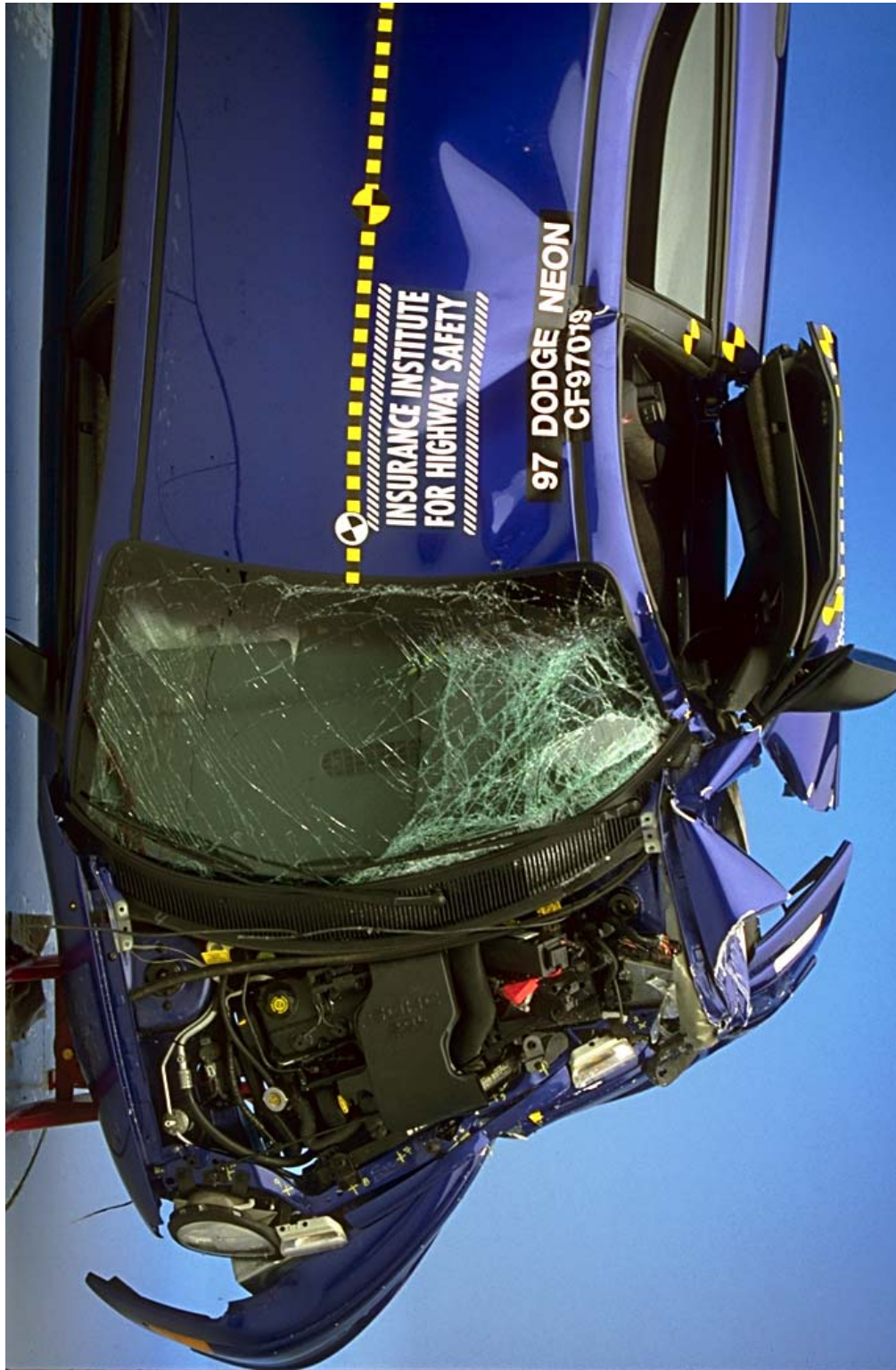
Figure 1 Overhead View of Crash Deformation — 1997 Dodge Neon
