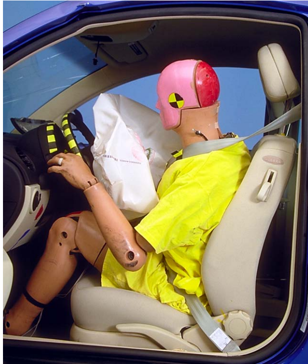
Figure 7 Dummy and Vehicle Interior, Postcrash — 1998 Volkswagen New Beetle
