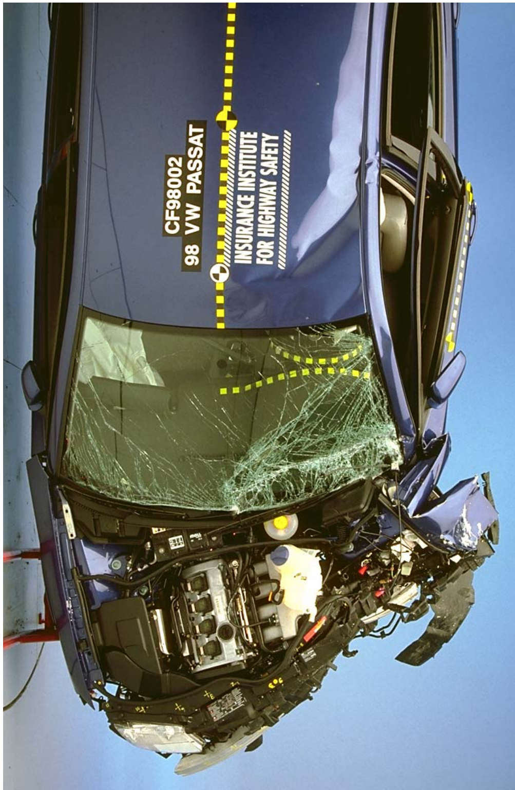
Figure 1 Overhead View of Crash Deformation — 1998 Volkswagen Passat
