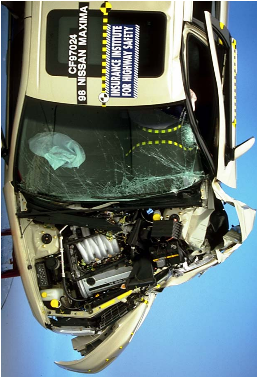
Figure 1 Overhead View of Crash Deformation — 1998 Nissan Maxima
