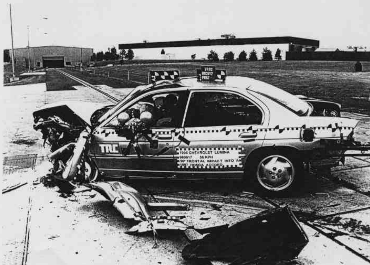
Figure A-22 Post-Test Bullet Vehicle Left Side View
