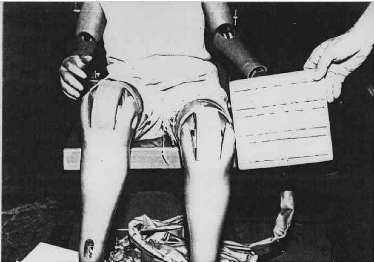
Figure A-88 Post-Test Bullet Vehicle Passenger Dummy Leg Contact - View 1
