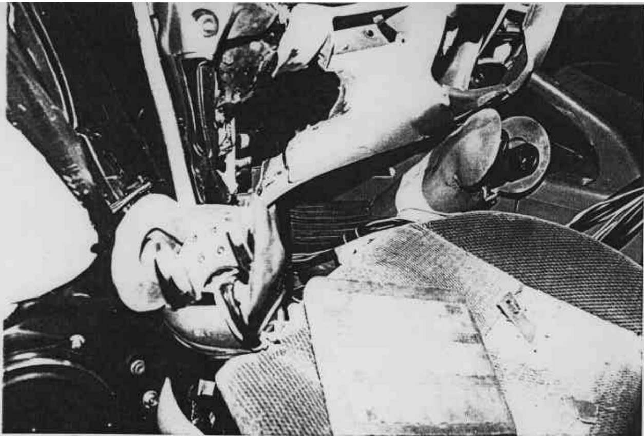
Figure A-68 Post-Test Target Vehicle Driver Dummy Knee Contact - View 3
