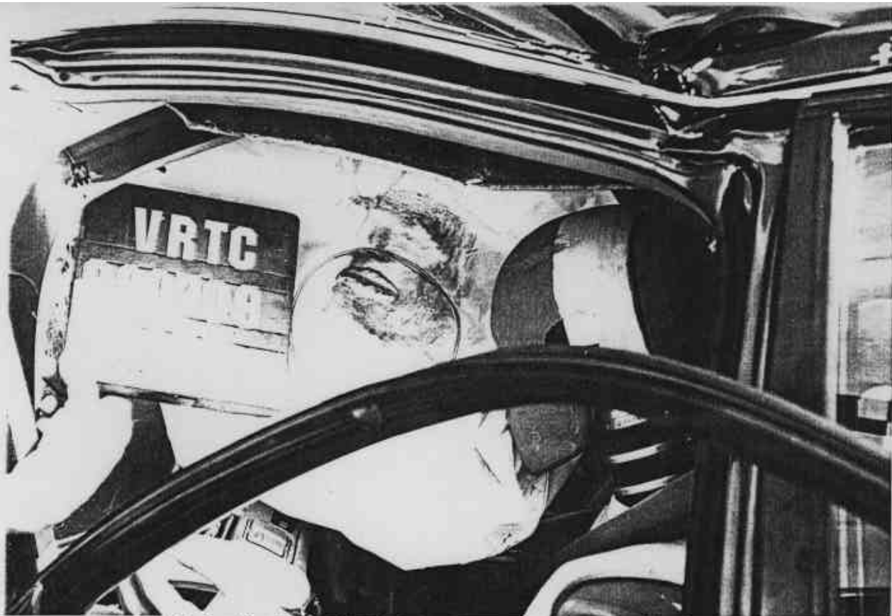
Figure A-64 Post-Test Target Vehicle Driver Dummy Head Contact - View 2
