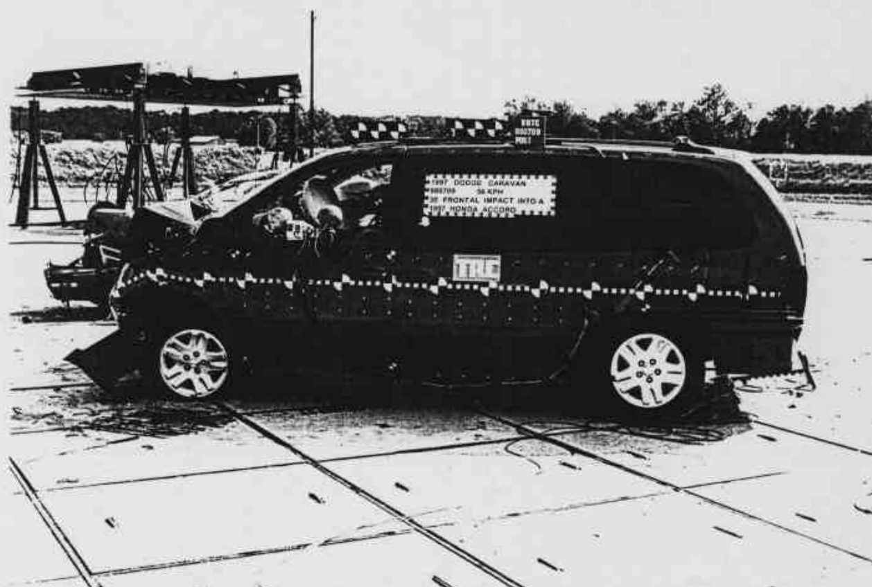
Figure A-25 Post-Test Bullet Vehicle Left Side View
