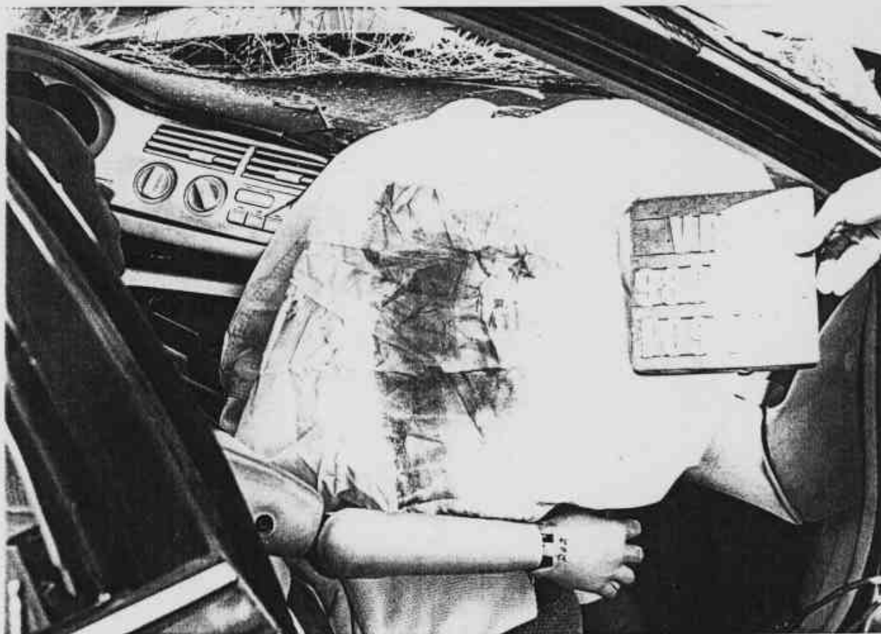
Figure A-71 Post-Test Target Vehicle Passenger Dummy Head Contact - View 2
