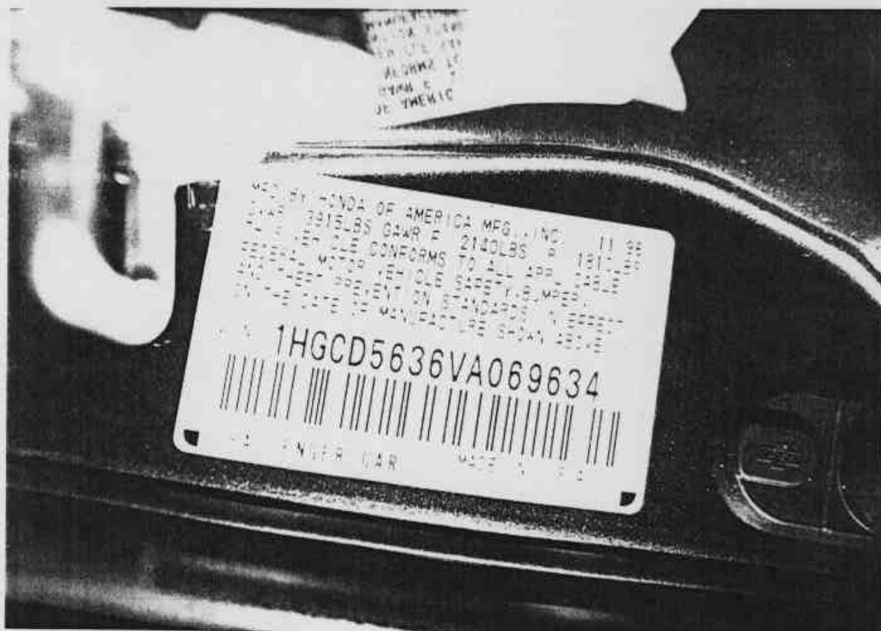
Figure A-91 Target Vehicle Certification Label
