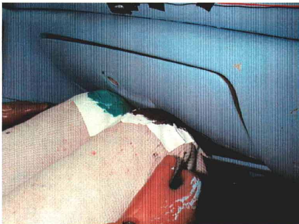
22. Point de contact, genoux du passager, après essai. Passenger's knees contact point, post-test.
