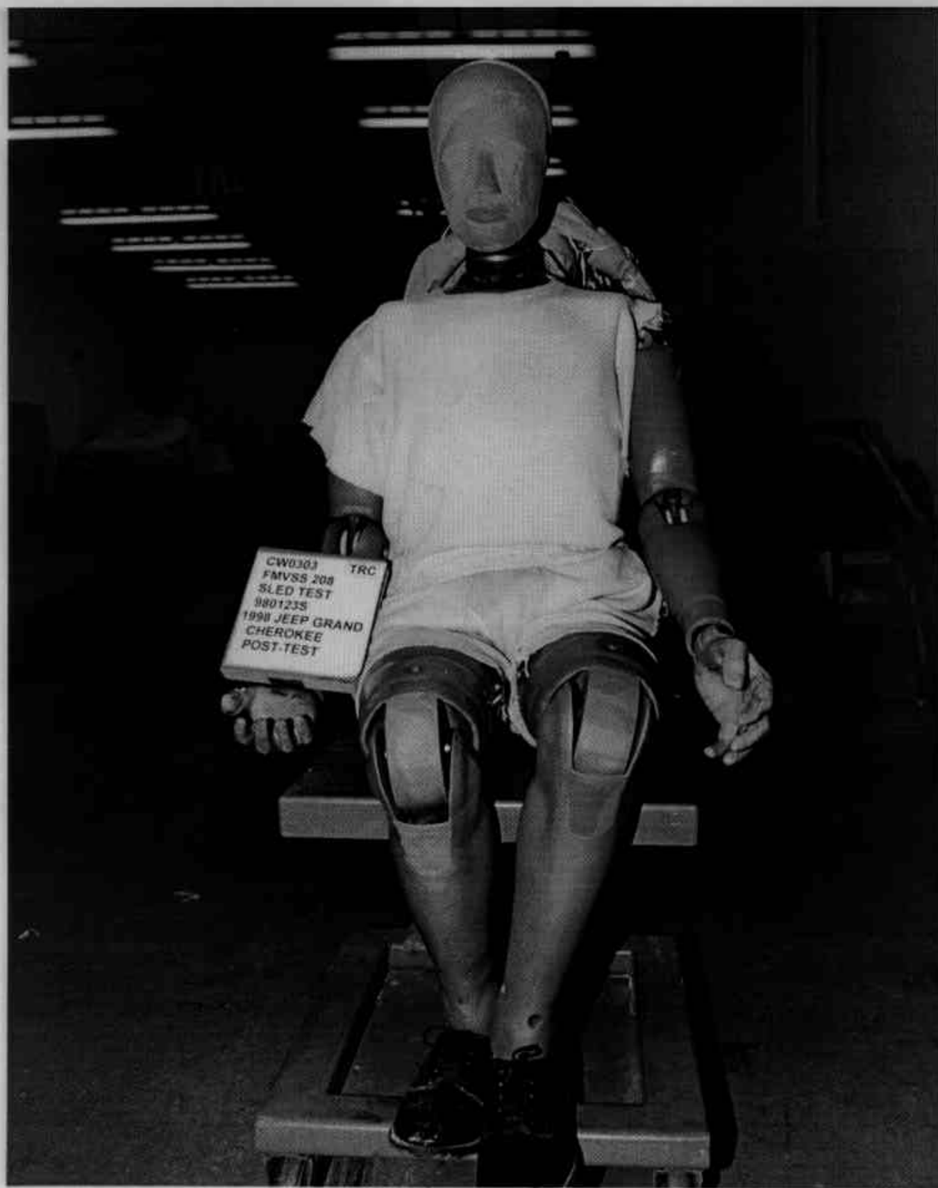
Figure A-18 Post-Test Driver Dummy Removed From Vehicle Overall View A-19 980123
