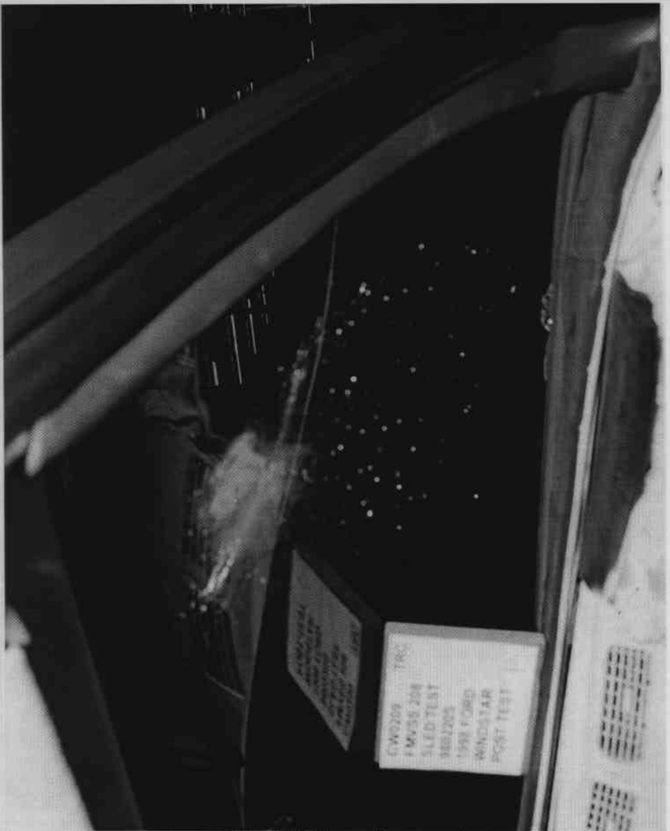
Figure A-30 Post-Test Passenger Head Contact View A-31
