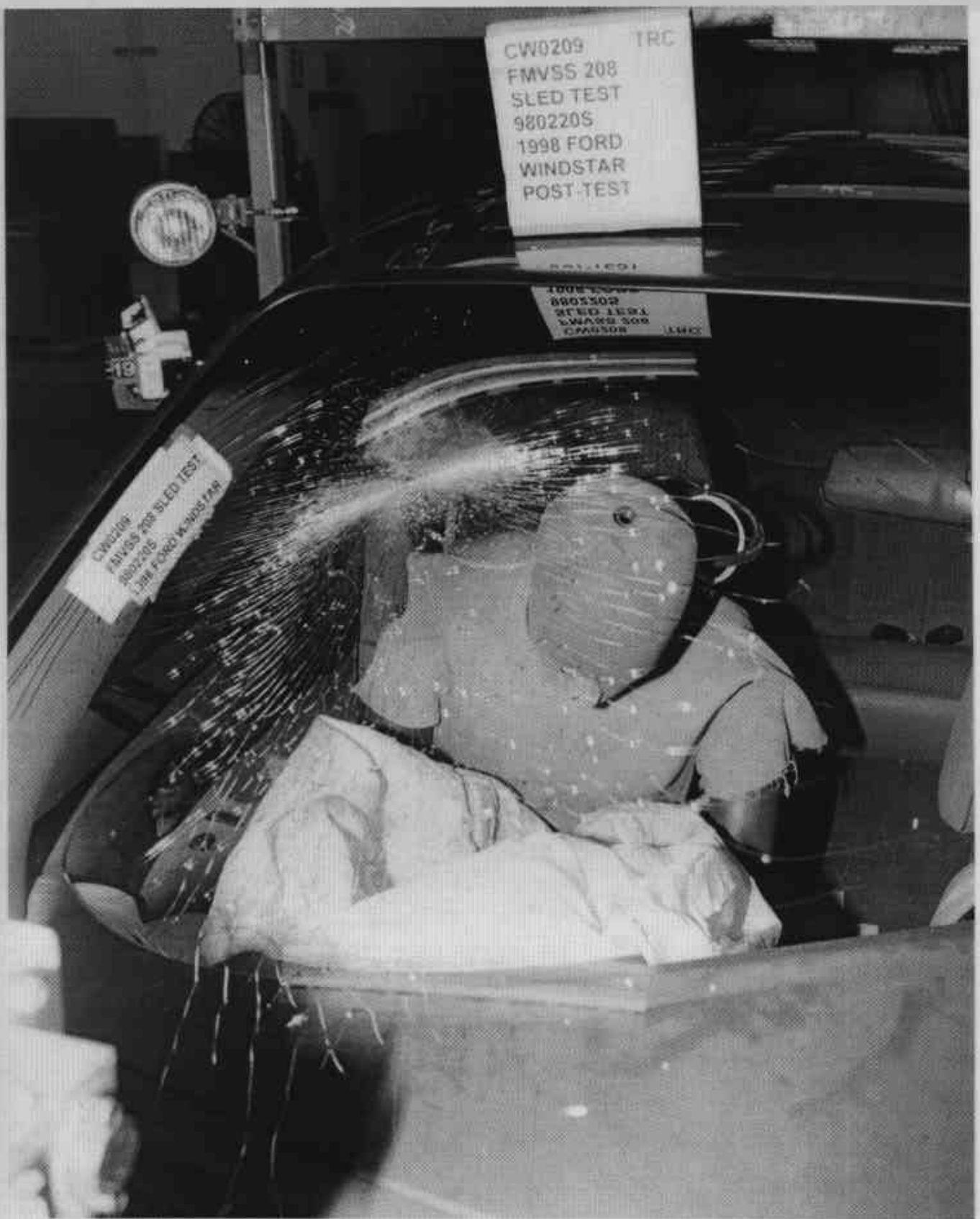
Figure A-27 Post-Test Passenger Dummy Position Front View
