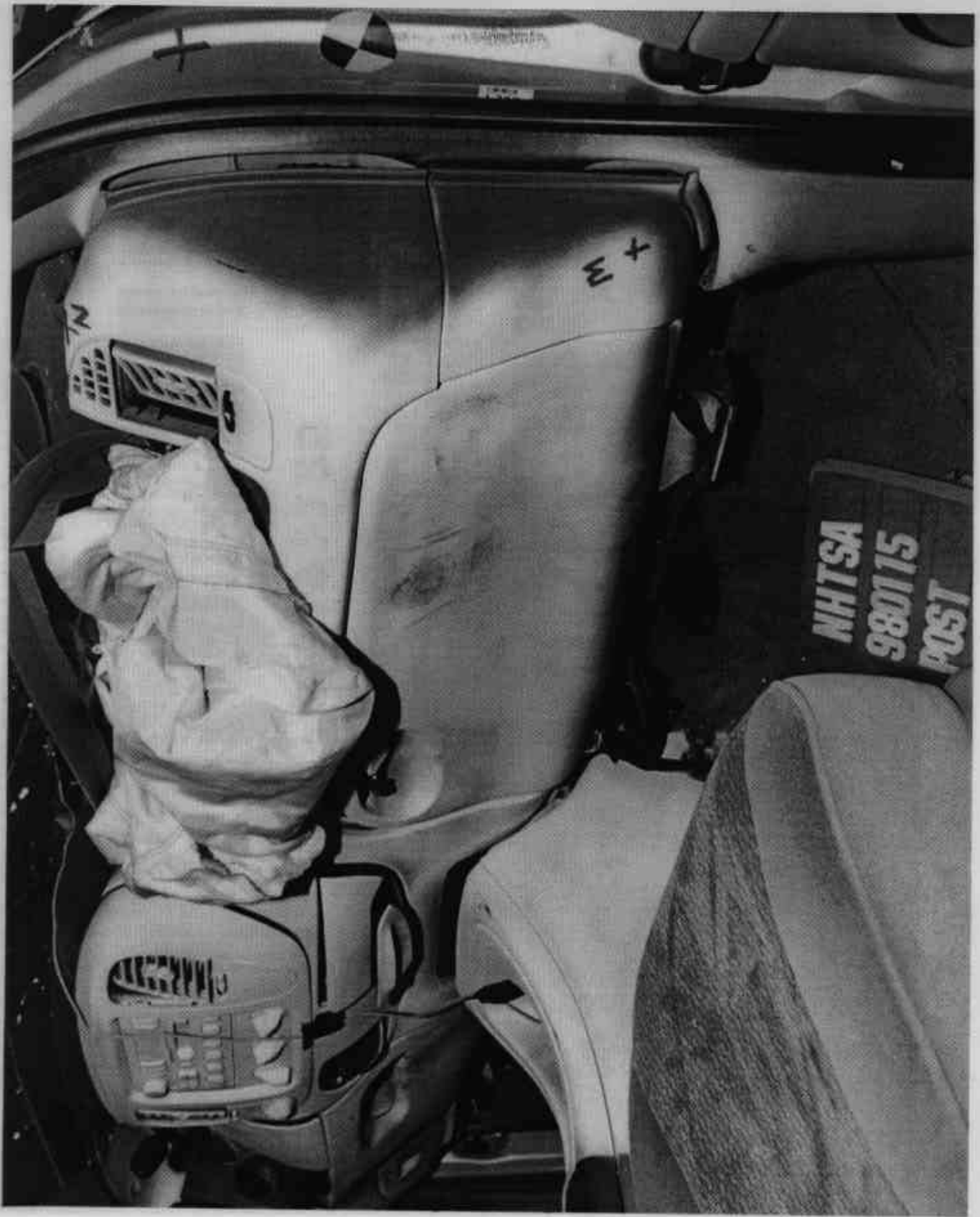
Figure A-51 Post-Test Passenger Dummy Knee Contact - View 2
