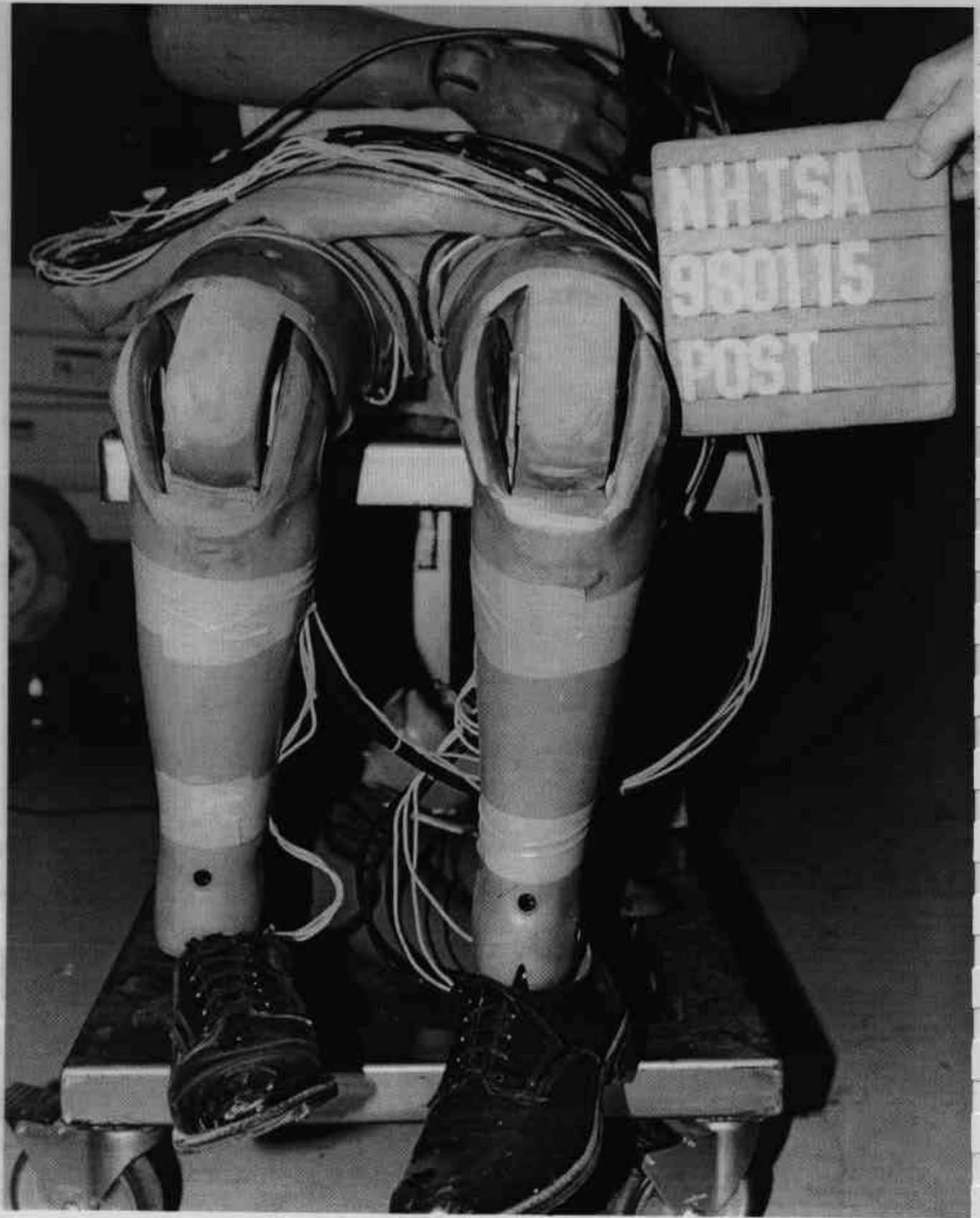
Figure A-50 Post-Test Passenger Dummy Knee Contact - View 1 A-51
