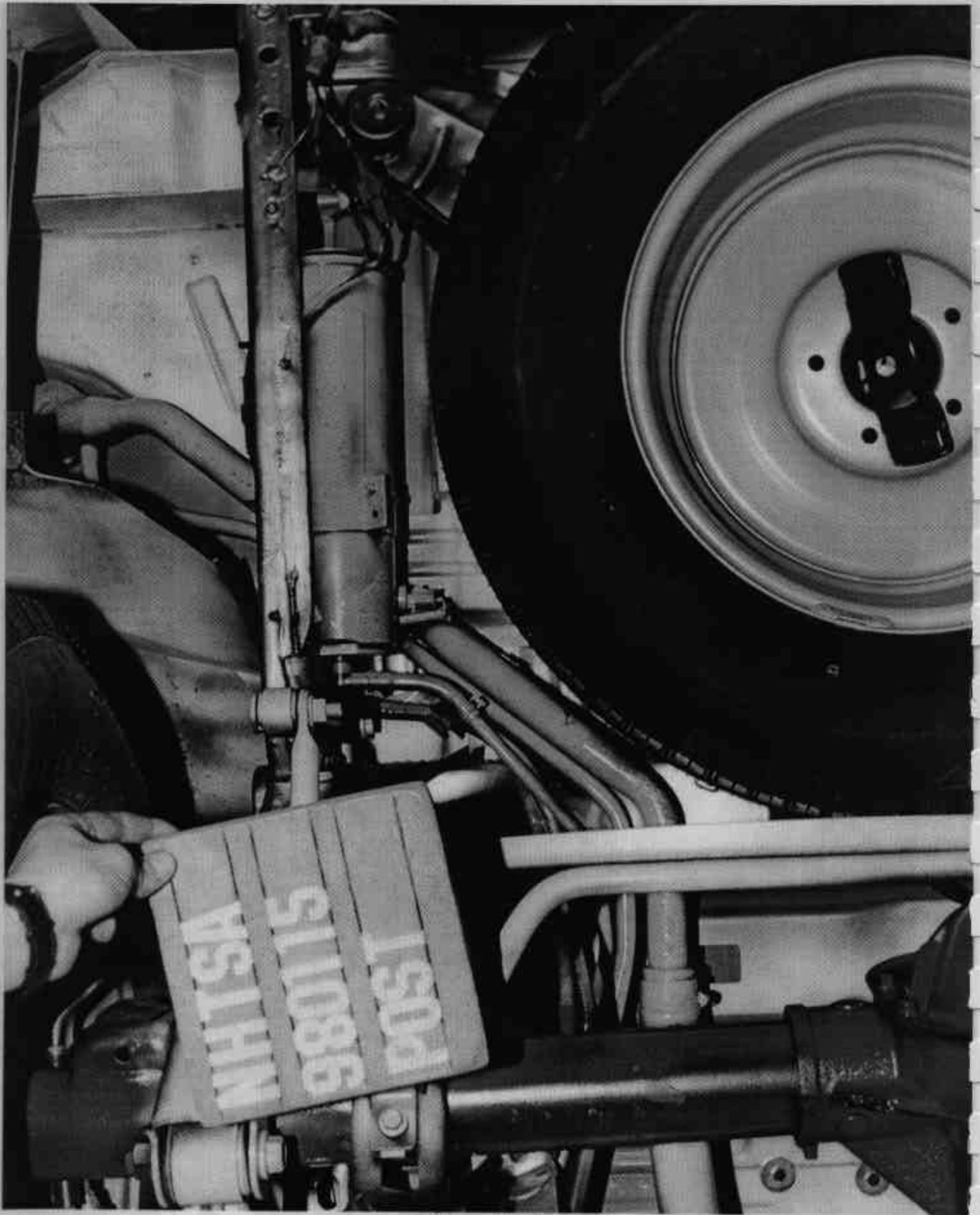
Figure A-20 Post-Test Fuel Filler Neck View
