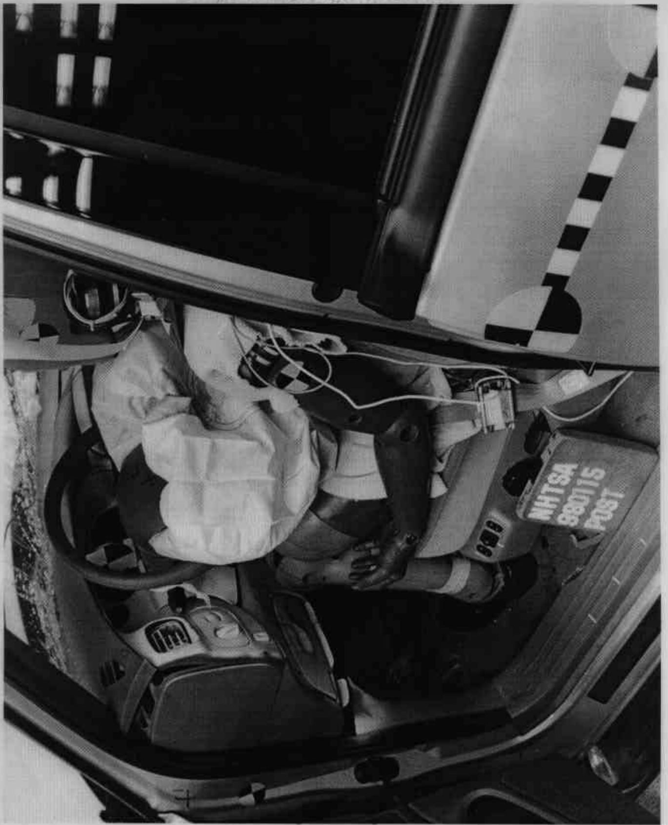
Figure A-35. Post-Test Driver Dummy and Vehicle Interior - View 2
