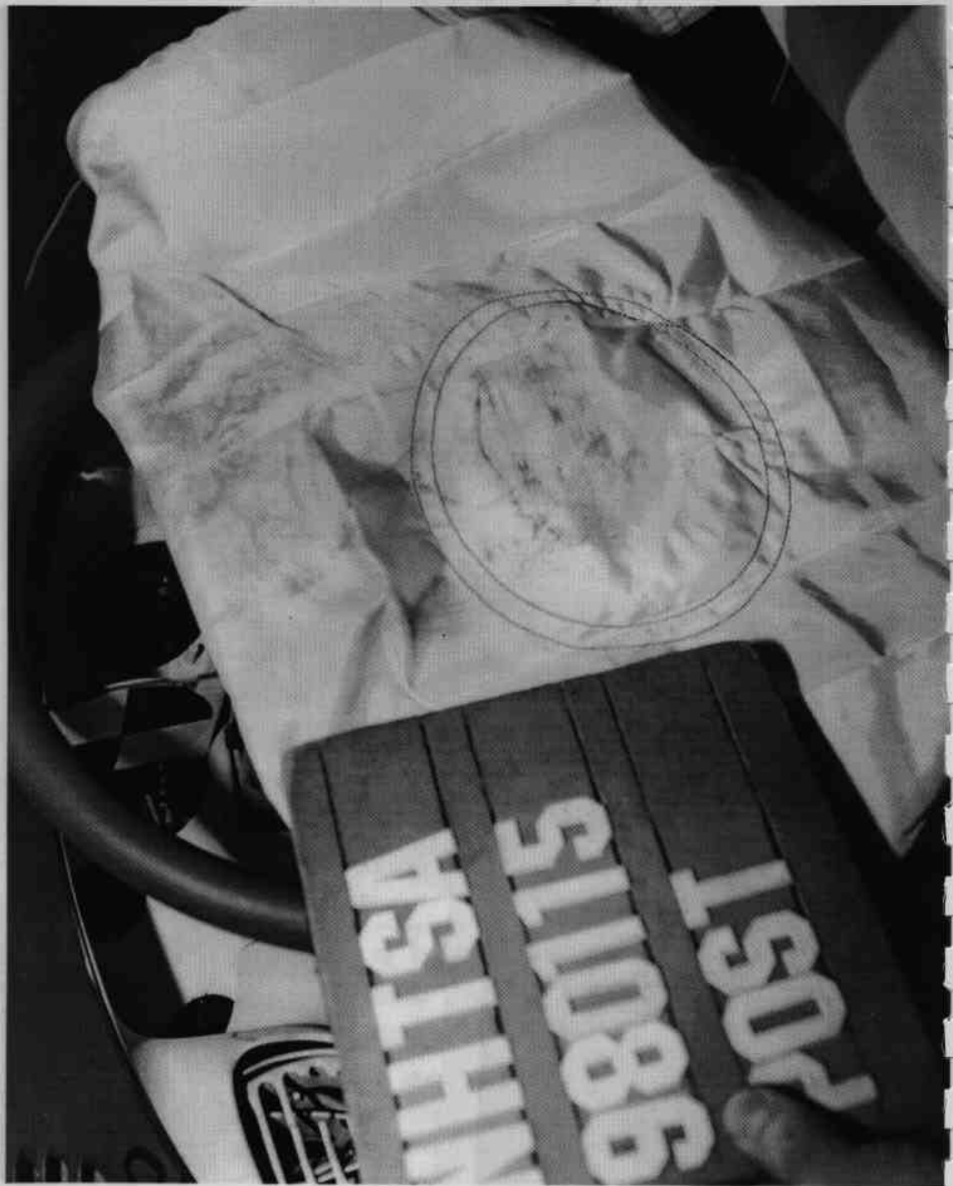
Figure A-42 Post-Test Driver Dummy Head Contact - View 2
