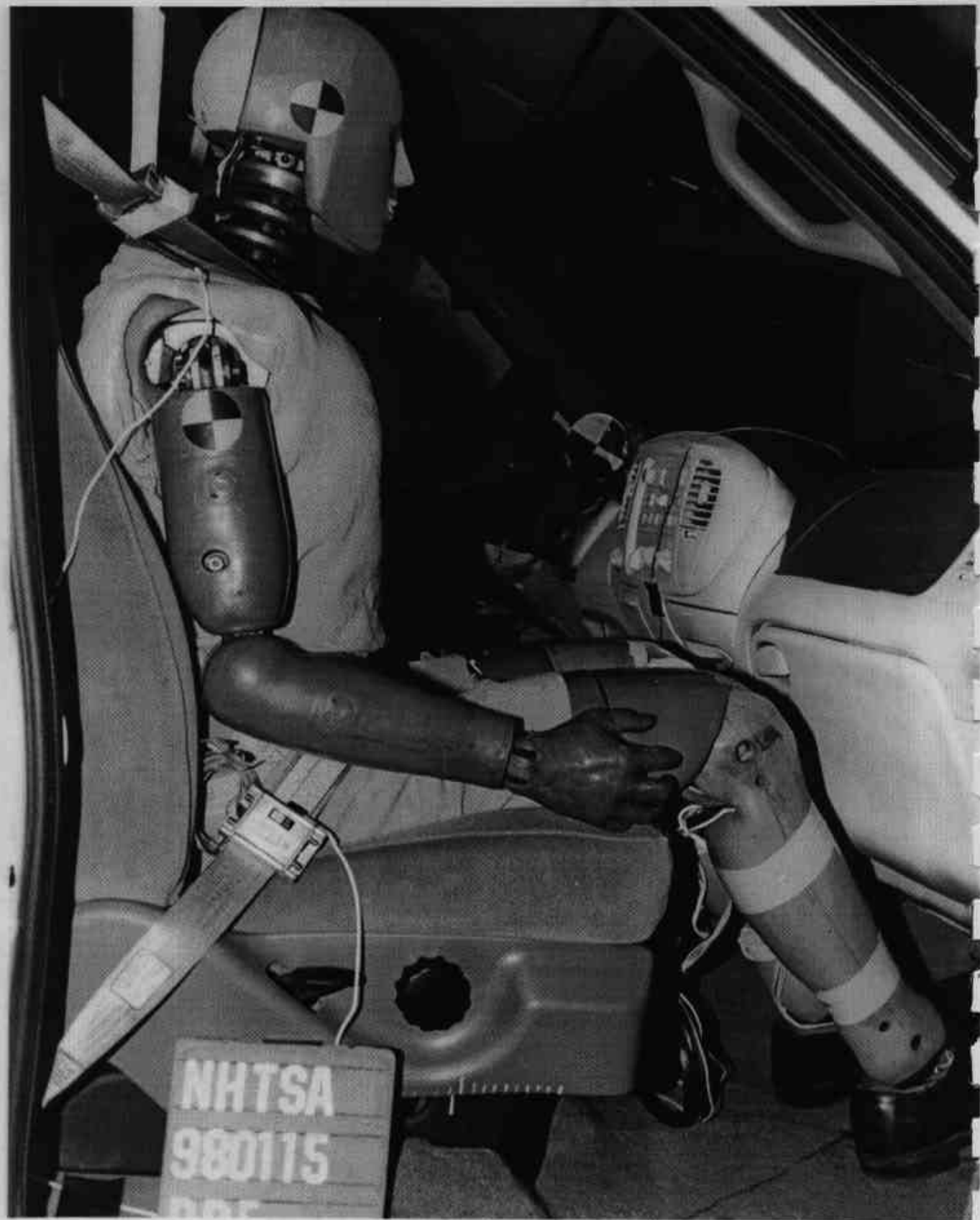
Figure A-36 Pre-Test Passenger Dummy and Vehicle Interior - View 1
