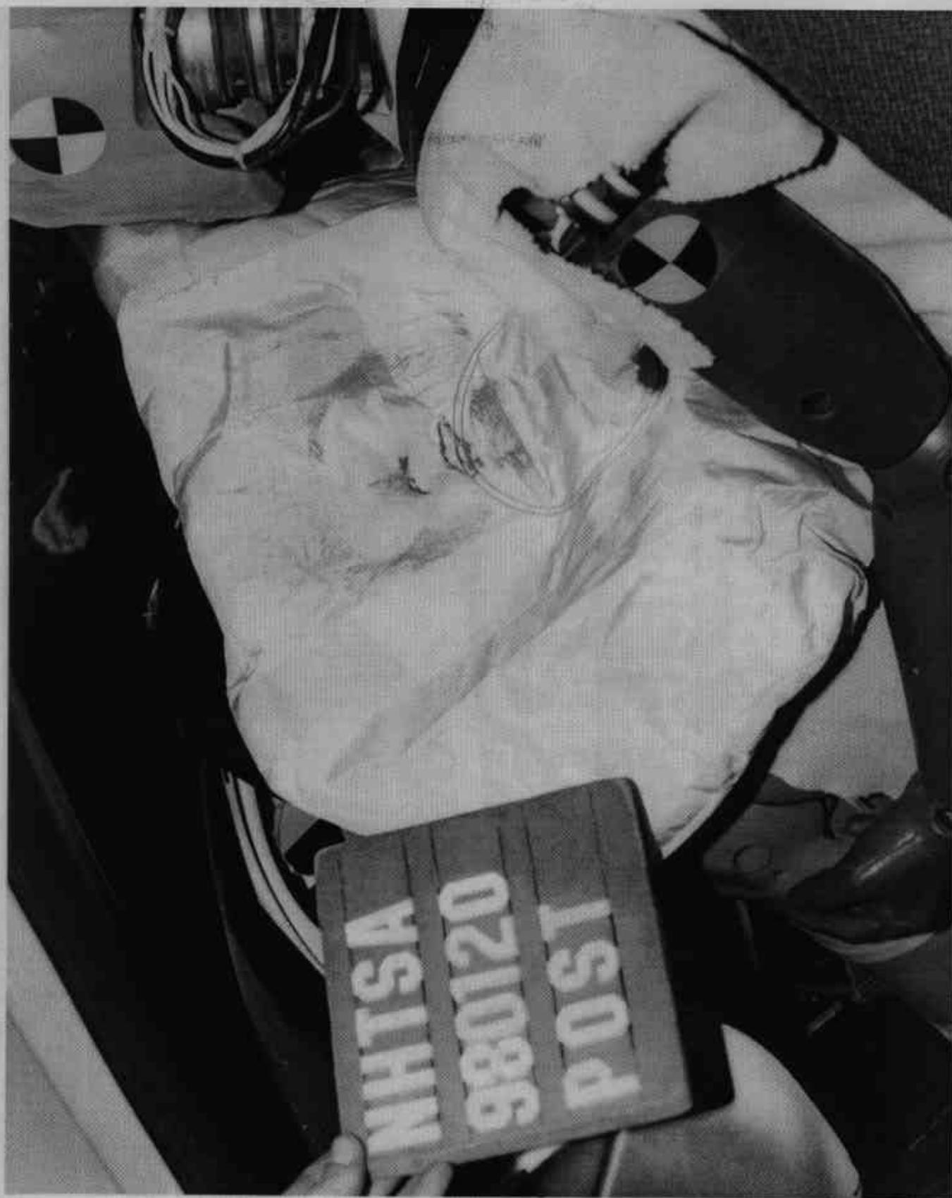
Figure A-41 Post-Test Driver Dummy Head Contact - View 2 A-42
