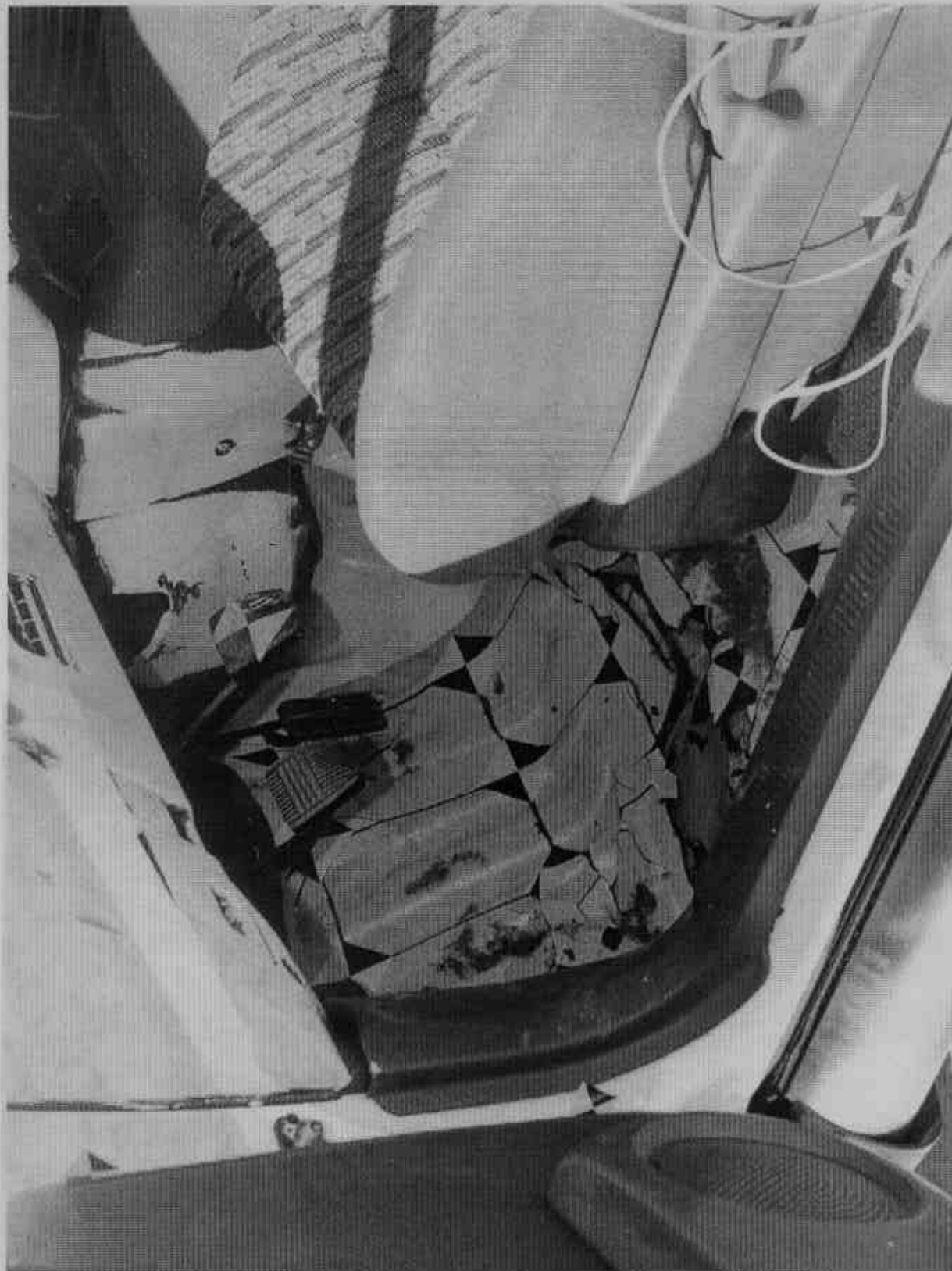
FIGURE A-26. POST TEST DRIVER FLOOR PAN
