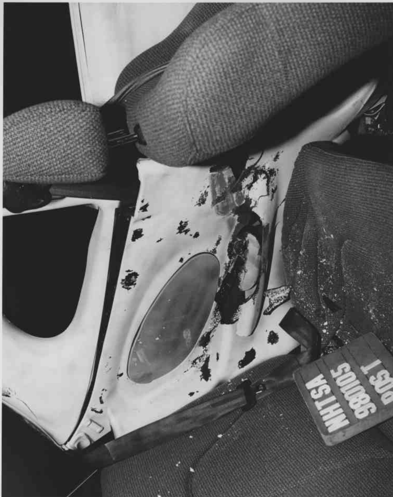
Figure A-28 Post-Test Interior Of Rear Panel Showing SID Impact Locations A-30 980105
