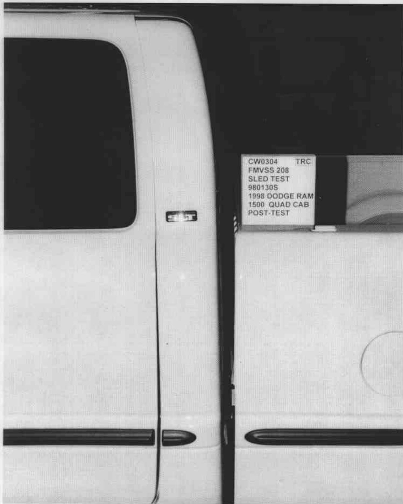
Figure A-35 Post-Test Vehicle Damage/Body Deformation - View 1
