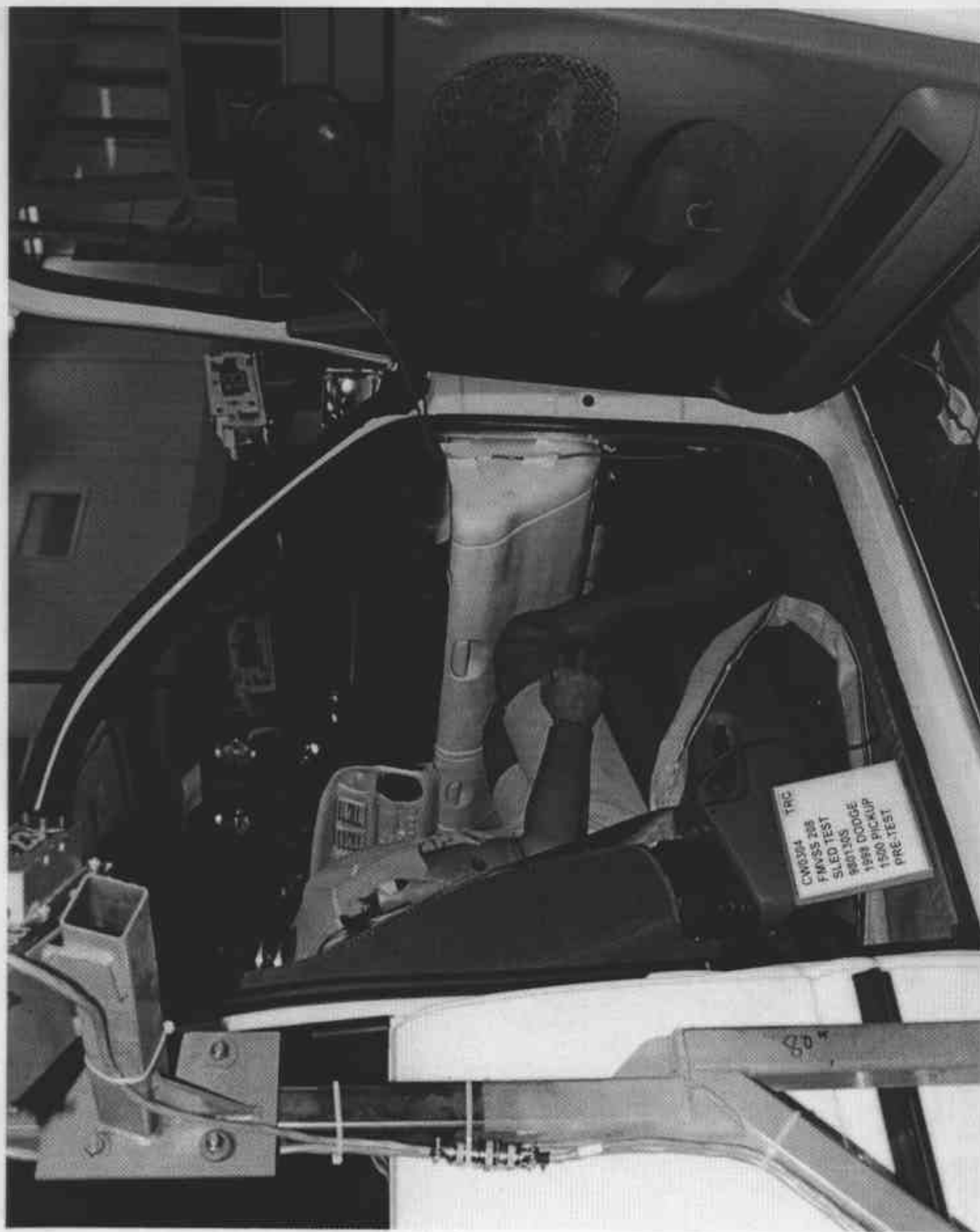
Figure A-21 Pre-Test Passenger Dummy Position View With Door Open - View 2 A-22 980130
