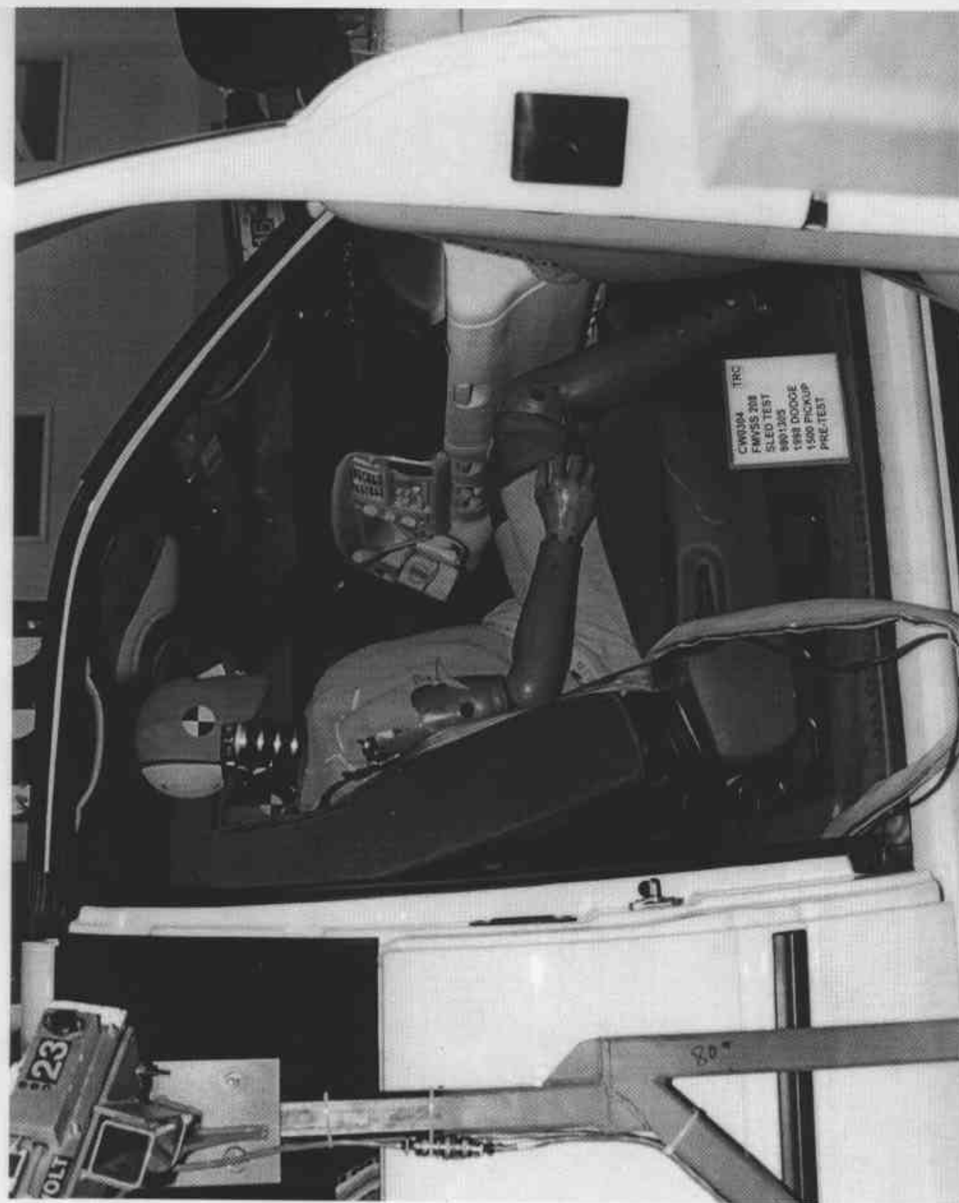
Figure A-19 Pre-Test Passenger Dummy Position View With Door Open - View 1 A-20 980130
