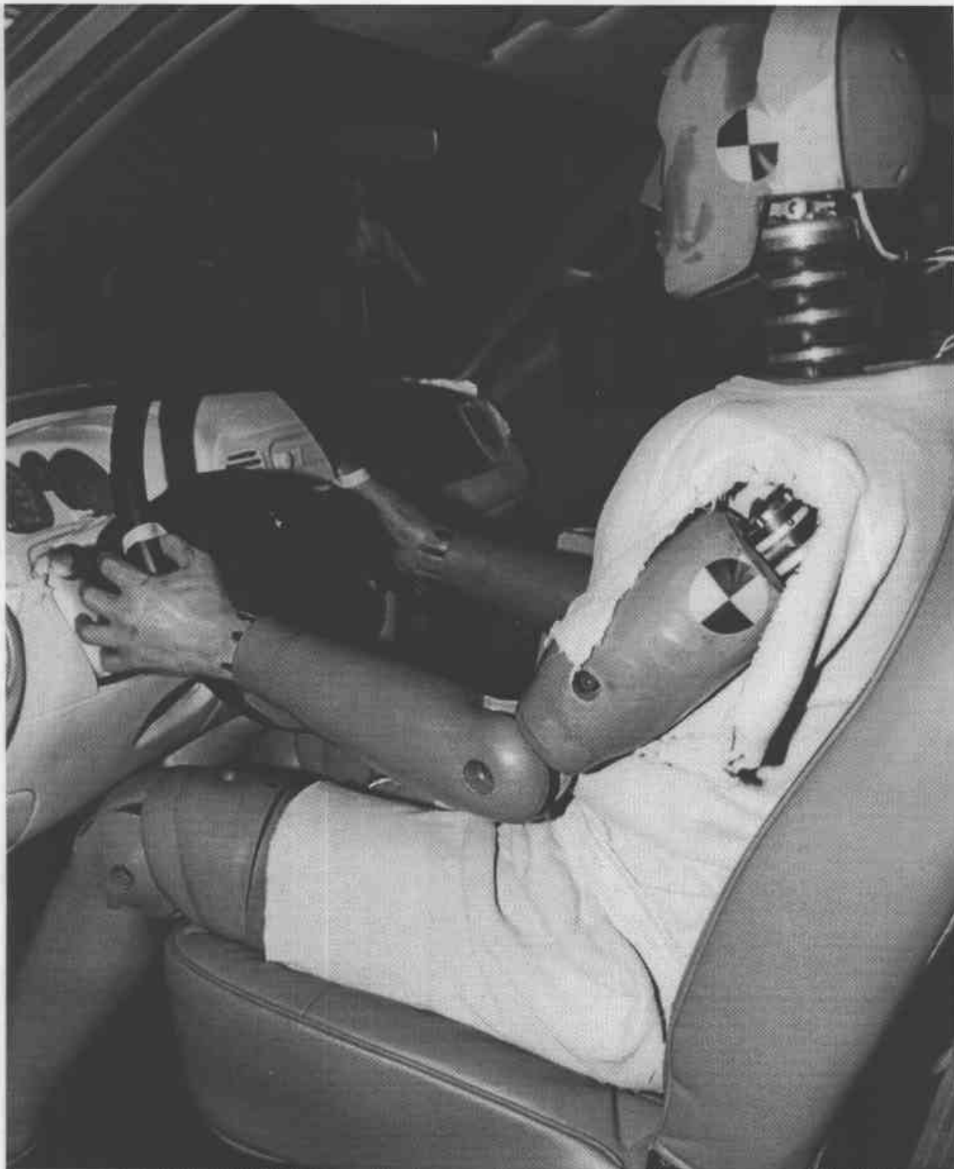
Figure A-6 Pre-Test Driver Dummy Position View With Door Open
