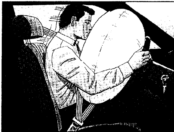
The right front passenger's air bag is in the instrument panel on the passenger's side.
