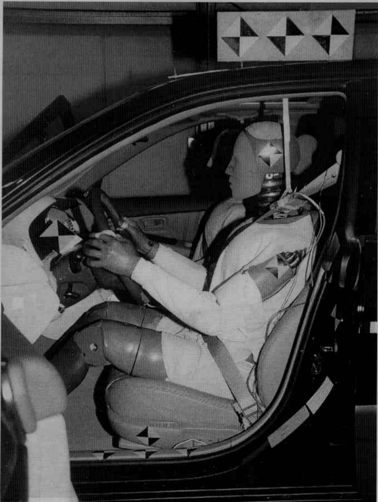
FIGURE A-33. PRETEST DRIVER DUMMY (90° TO VEHICLE)
