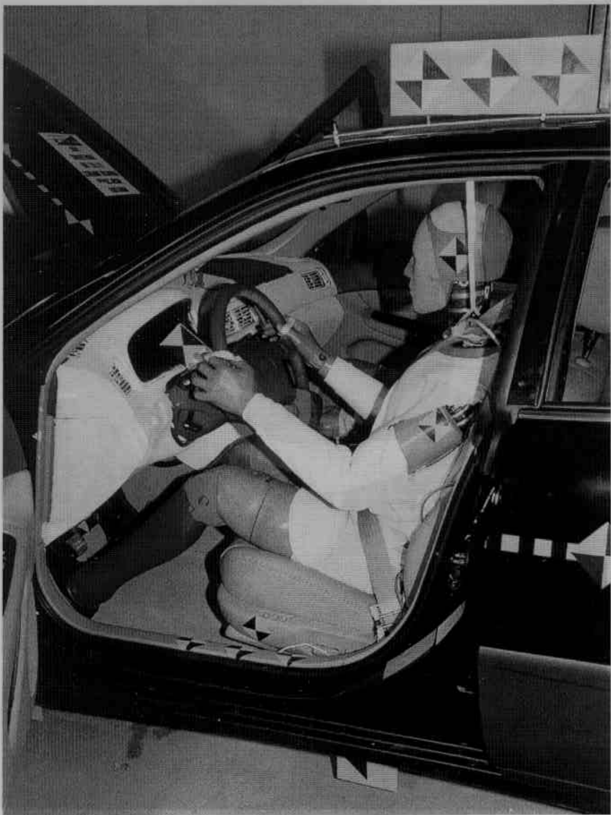
FIGURE A-31. PRETEST DRIVER DUMMY (DOOR OPEN)
