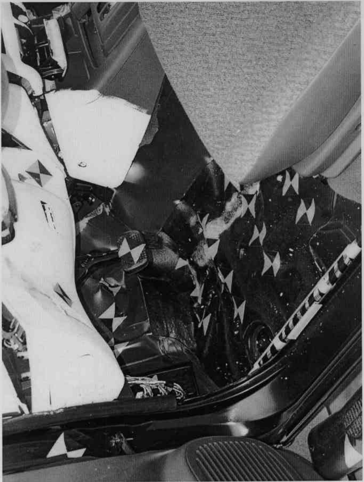
FIGURE A-26. POST TEST DRIVER FLOOR PAN
