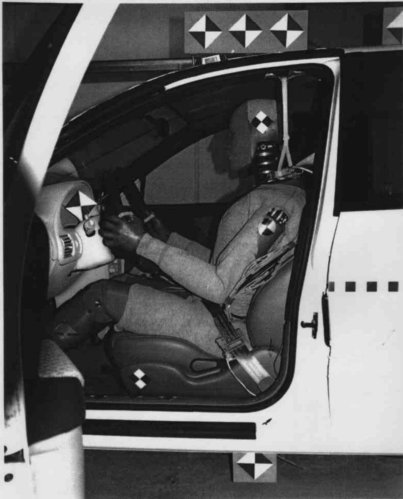
FIGURE A-31. PRETEST DRIVER DUMMY (90° TO VEHICLE)
