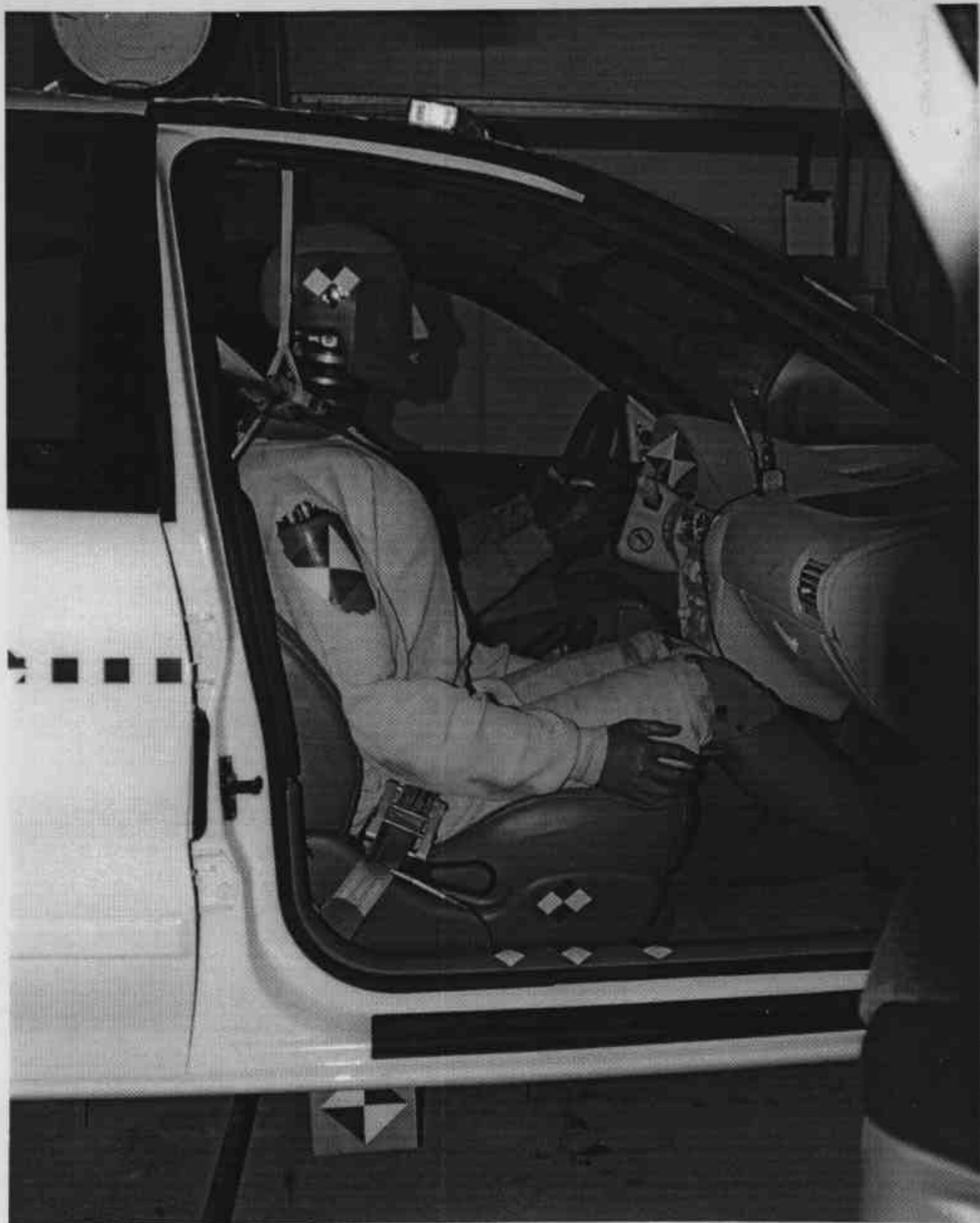
FIGURE A-44. PRE-TEST PASSENGER DUMMY (90° TO VEHICLE)
