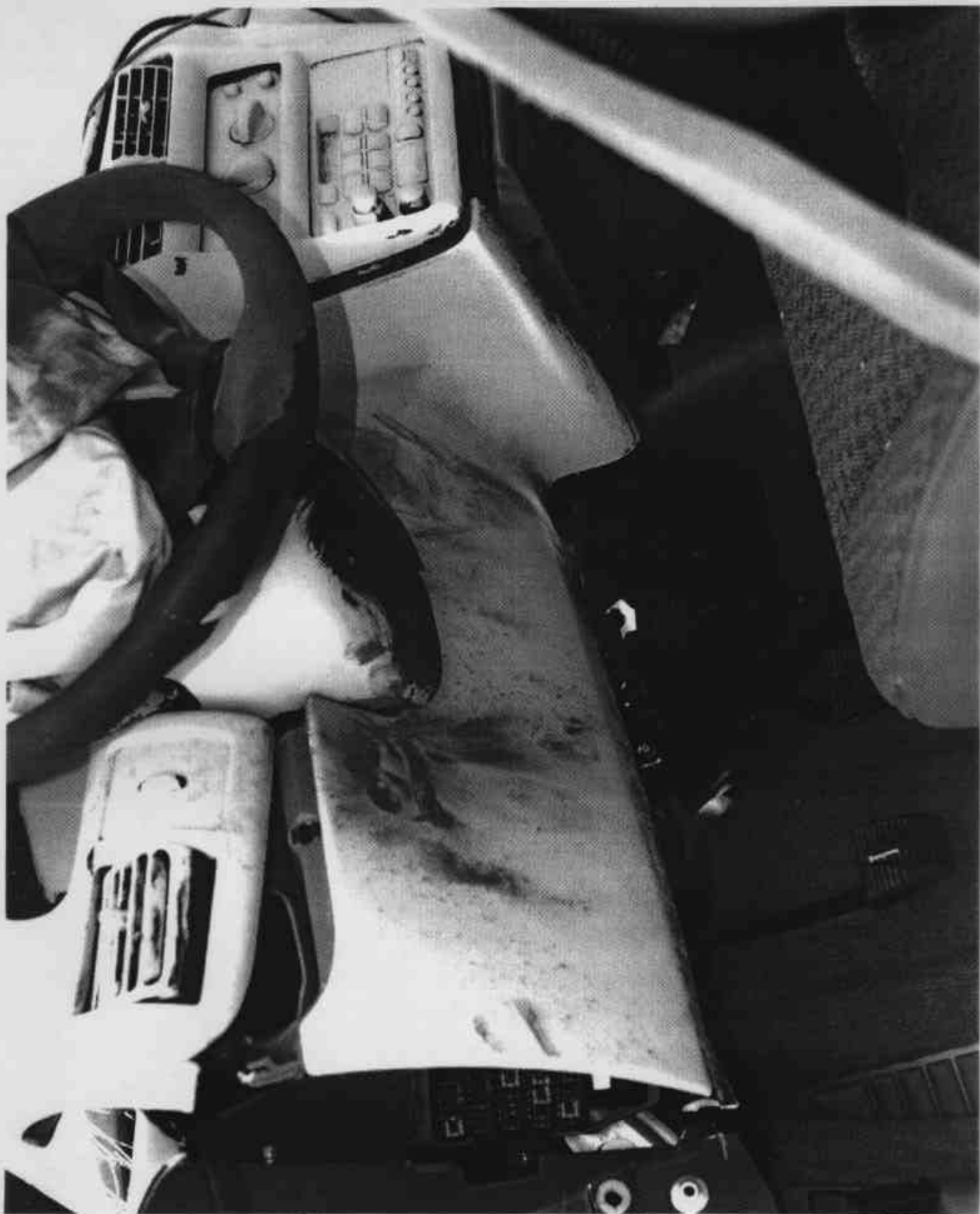
FIGURE A-37. POST-TEST DRIVER SIDE KNEE BOLSTER
