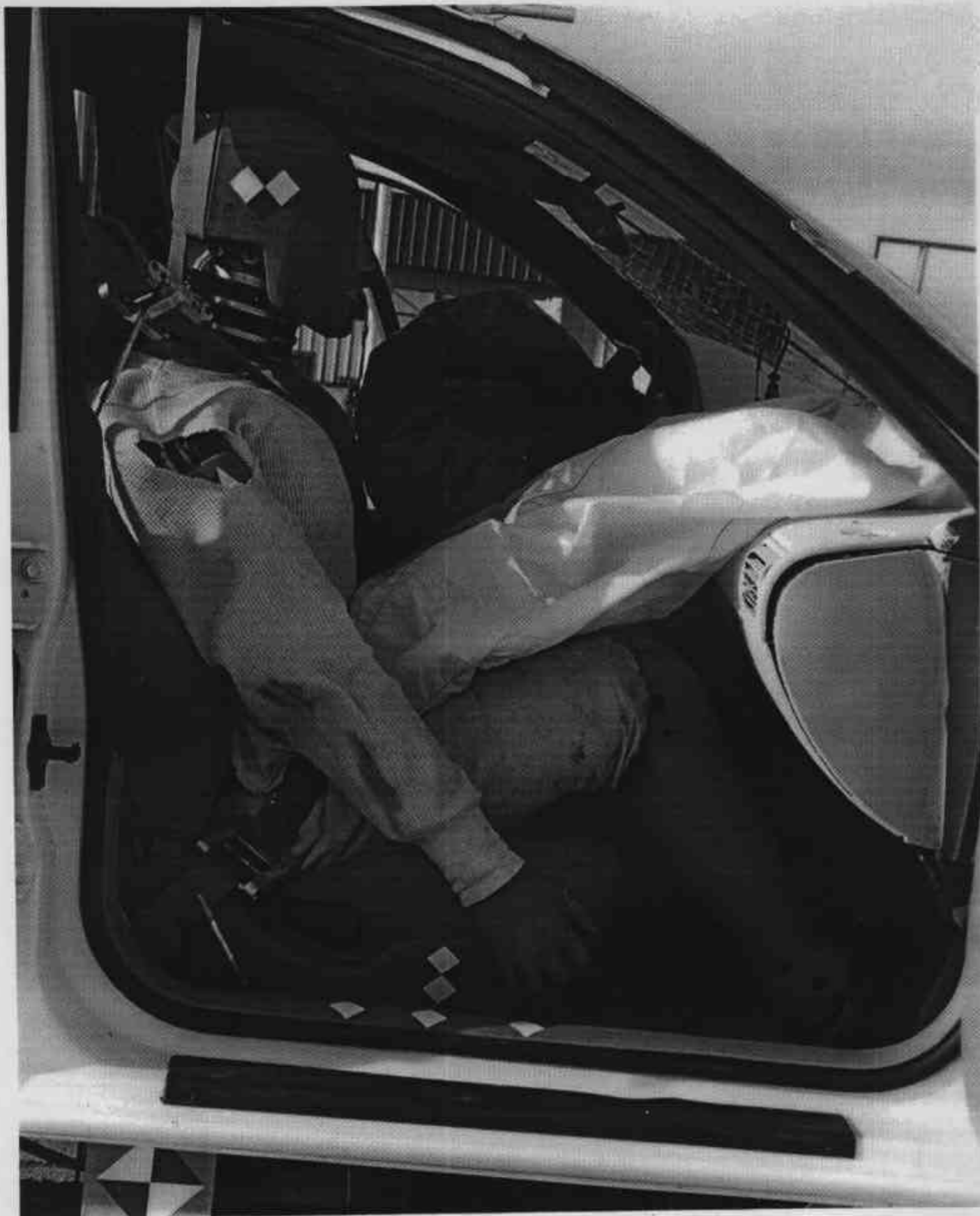
FIGURE A-45. POST-TEST PASSENGER DUMMY (90° TO VEHICLE)
