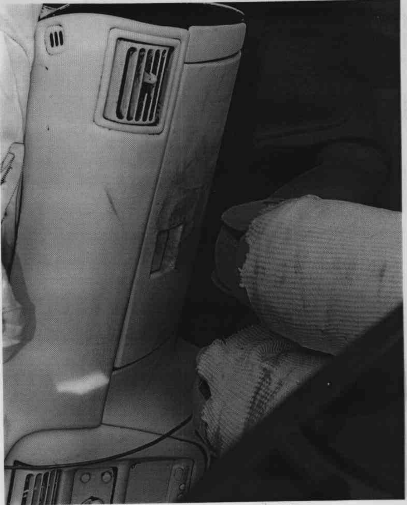
FIGURE A-48. POST-TEST PASSENGER DUMMY CONTACT POINTS (3 OF 3)
