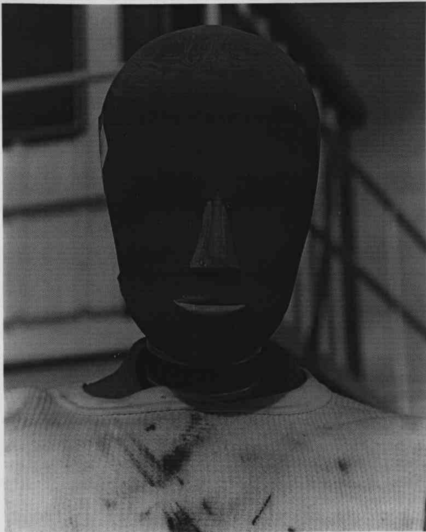
FIGURE A-46. POST-TEST PASSENGER DUMMY CONTACT POINTS (1 OF 3)
