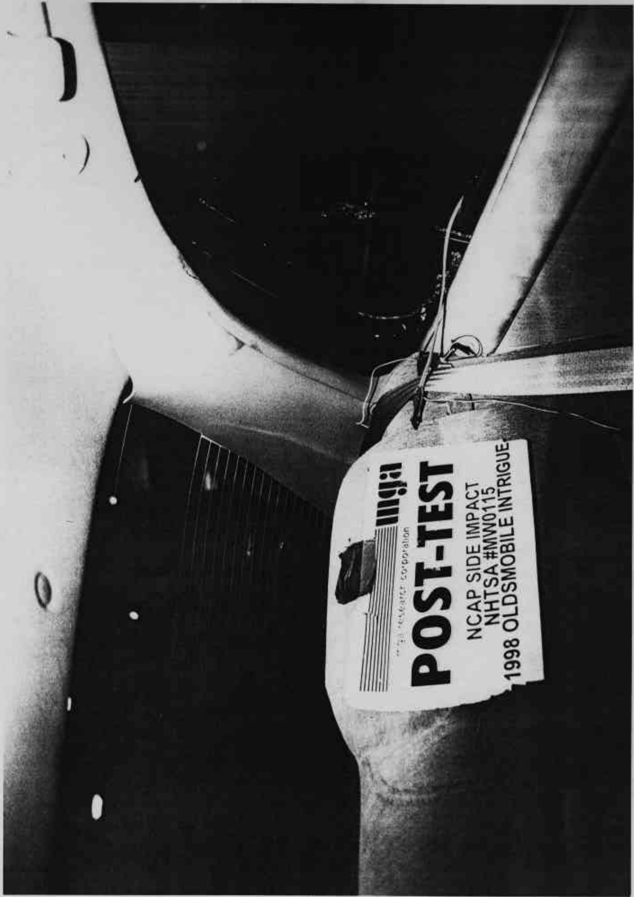
Photo No. A-38 - Post-Test Passenger Dummy Head Contact
