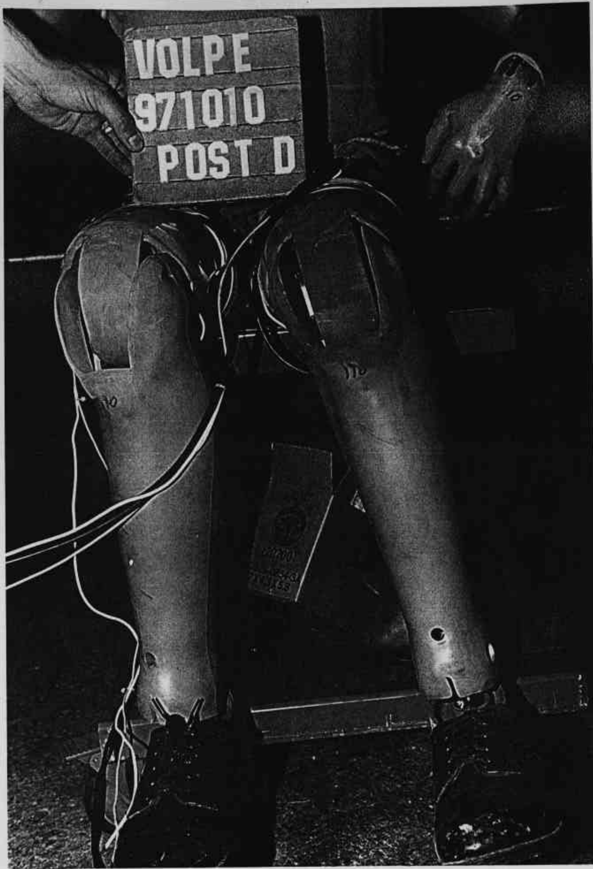
Figure A-43 Post-Test Driver Dummy Knee Contact - View 1
