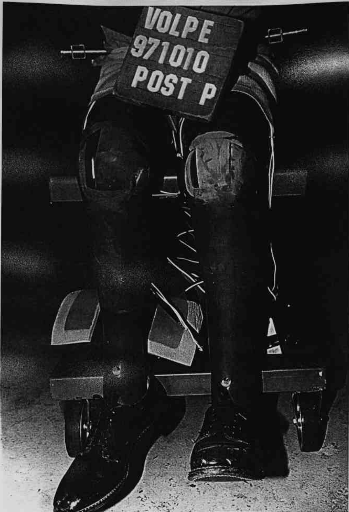
Figure A-49 Post-Test Passenger Dummy Knee Contact - View 1
