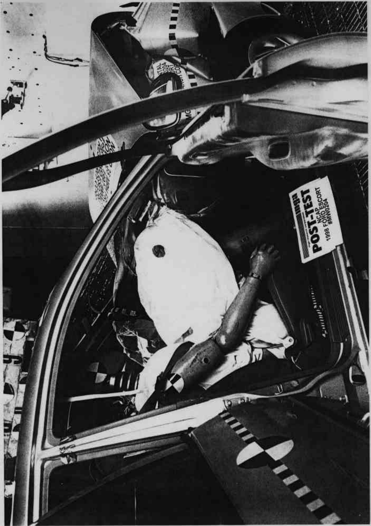
Photo No. A-35 - Post-Test Passenger Dummy Position Right Side View (Door Open)
