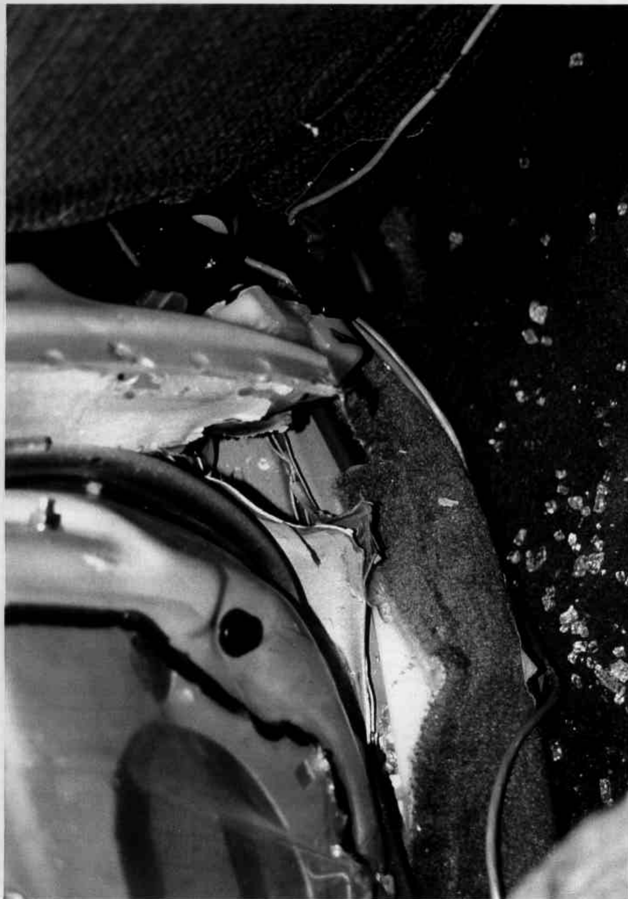
Figure A-36 POST-TEST CLOSEUP OF LOWER B-PILLAR
