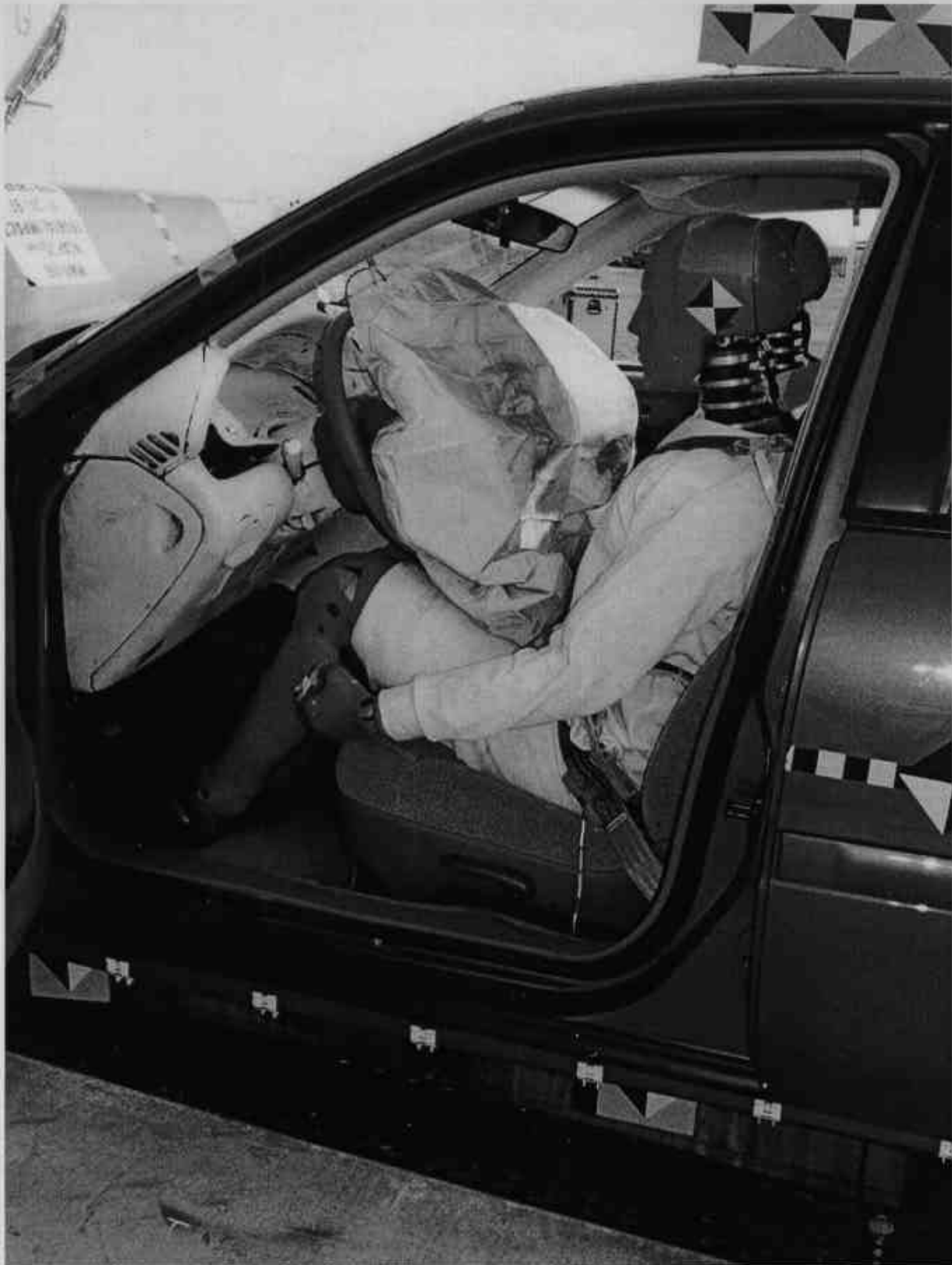
FIGURE A-32. POST TEST DRIVER DUMMY (DOOR OPEN)
