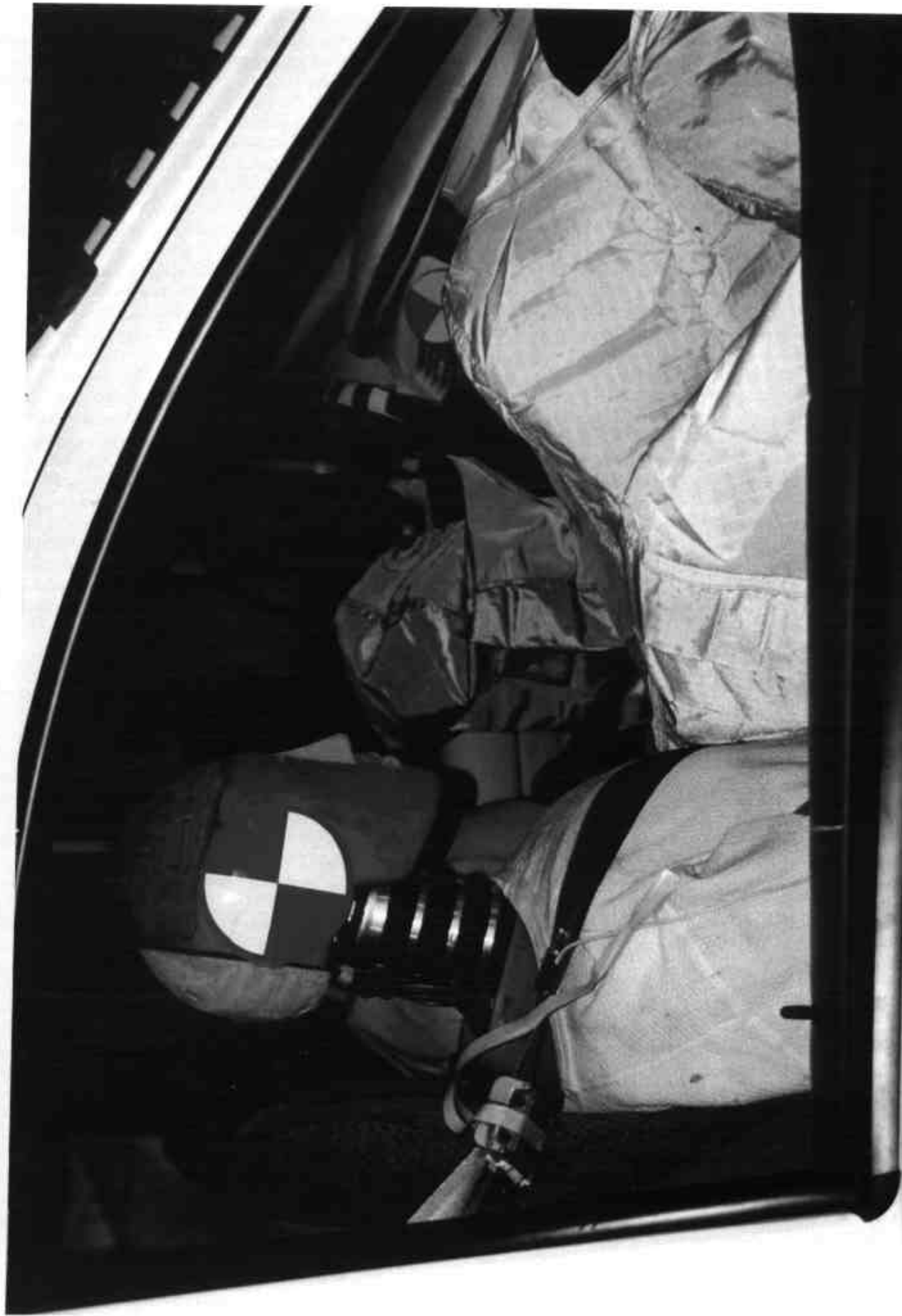
Figure A-33 POST-TEST PASSENGER HEAD LOCATION
