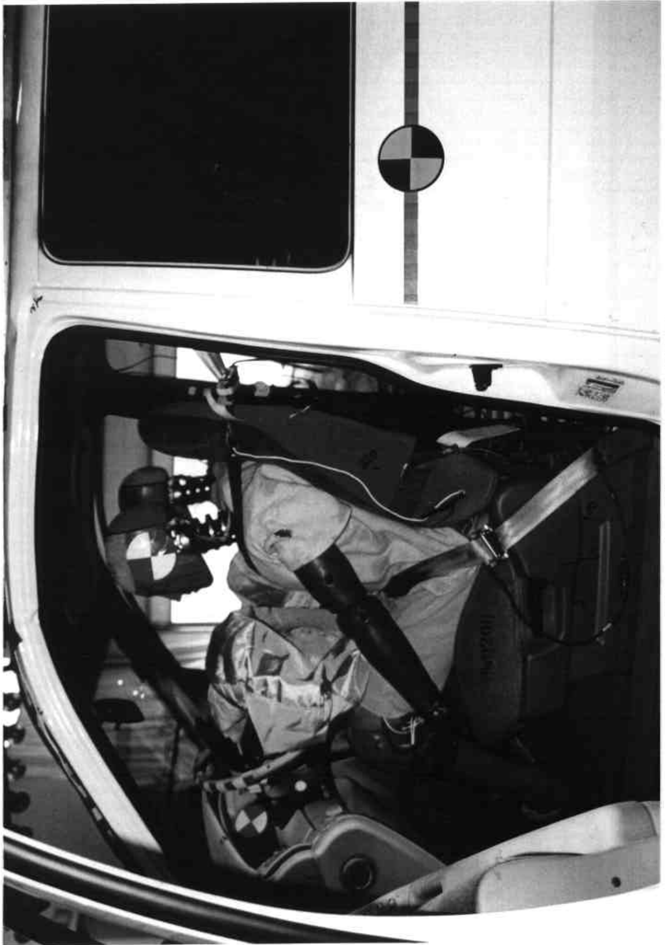
Figure A-23 POST-TEST DRIVER POSITION VIEW
