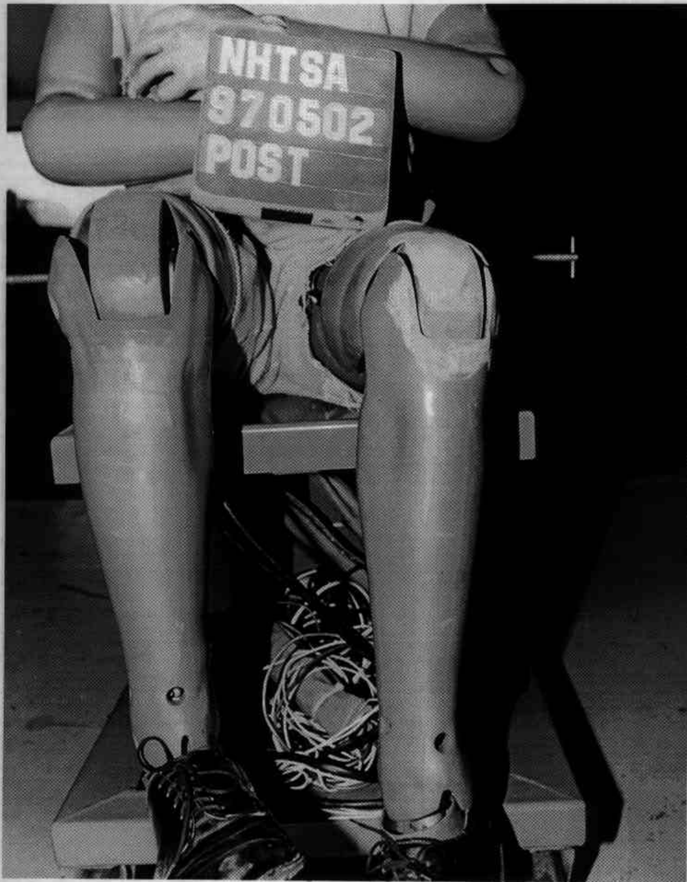
Figure A-45 Post-Test Passenger Dummy Knee Contact - View 1
