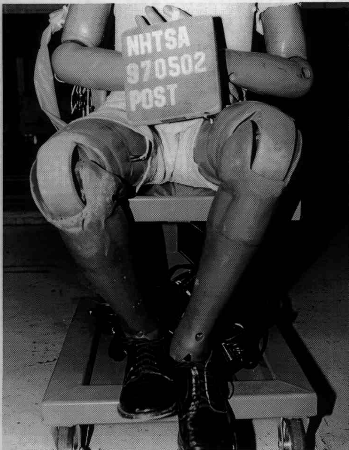
Figure A-41 Post-Test Driver Dummy Knee Contact - View 1 A-42
