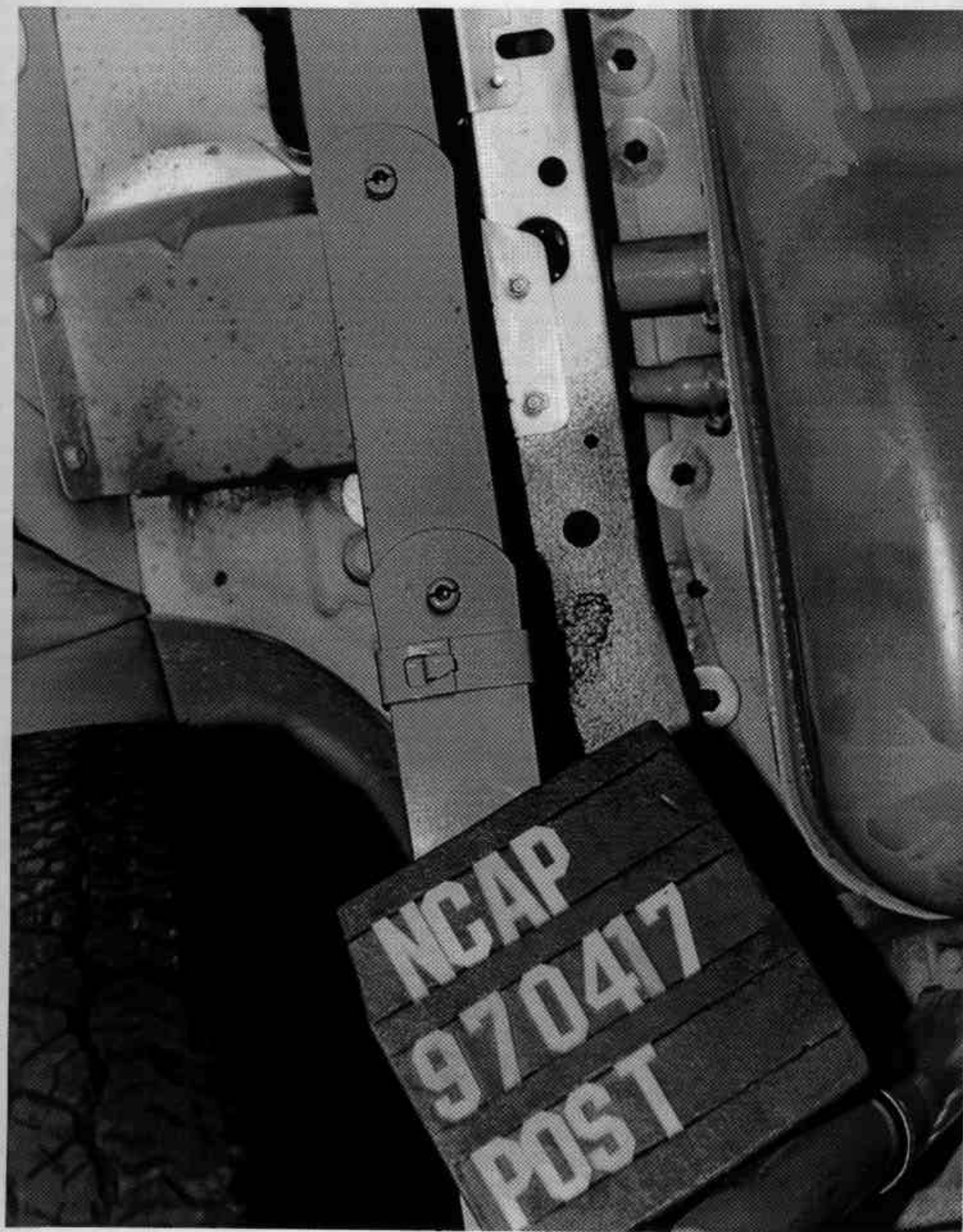
Figure A-19 Post-Test Fuel Filler Neck View A-20
