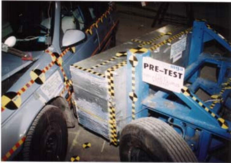
Photo No. A-7 - Pre-Test MDB Positioned Against Vehicle (left side)
