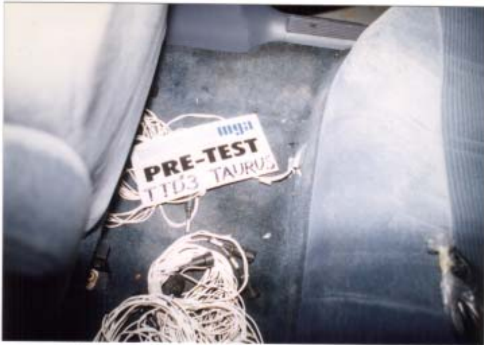
Photo No. A-59 - Pre-Test Rear Occupant Accelerometer
