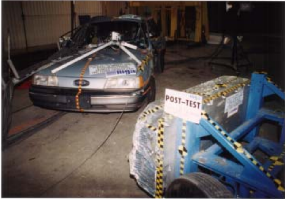
Photo No. A-10 - Post-Test MDB Positioned Against Vehicle (left side)
