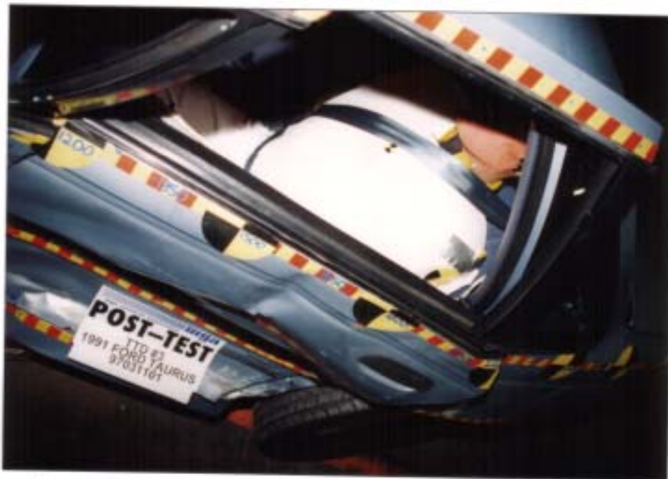
Photo No. A-37 - Post-Test Rear Passenger Dummy Shoulder and Door Top View
