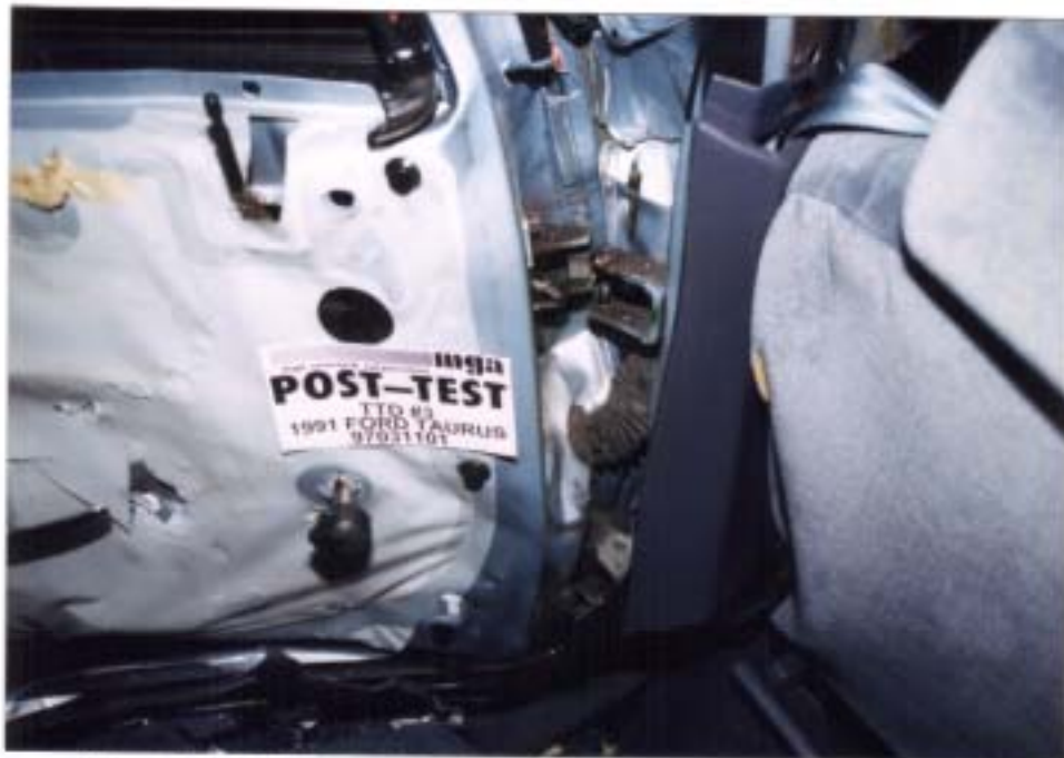
Photo No. A-62 - Post-Test Rear Door Upper Hinge Pin Failure
