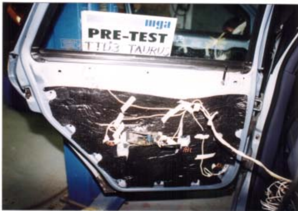
Photo No. A-60 - Pre-Test Rear Door Accelerometer Locations
