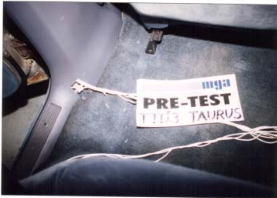
Photo No. A-57 - Pre-Test Left Lower B-Post Accelerometer
