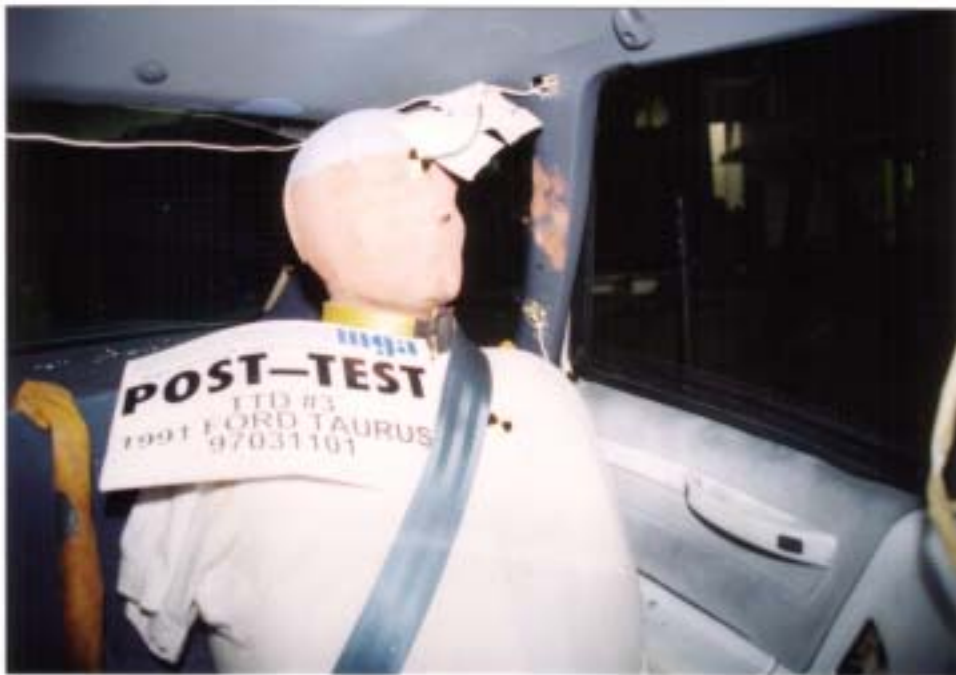
Photo No. A-39 - Post-Test Rear Passenger Dummy Head Contact
