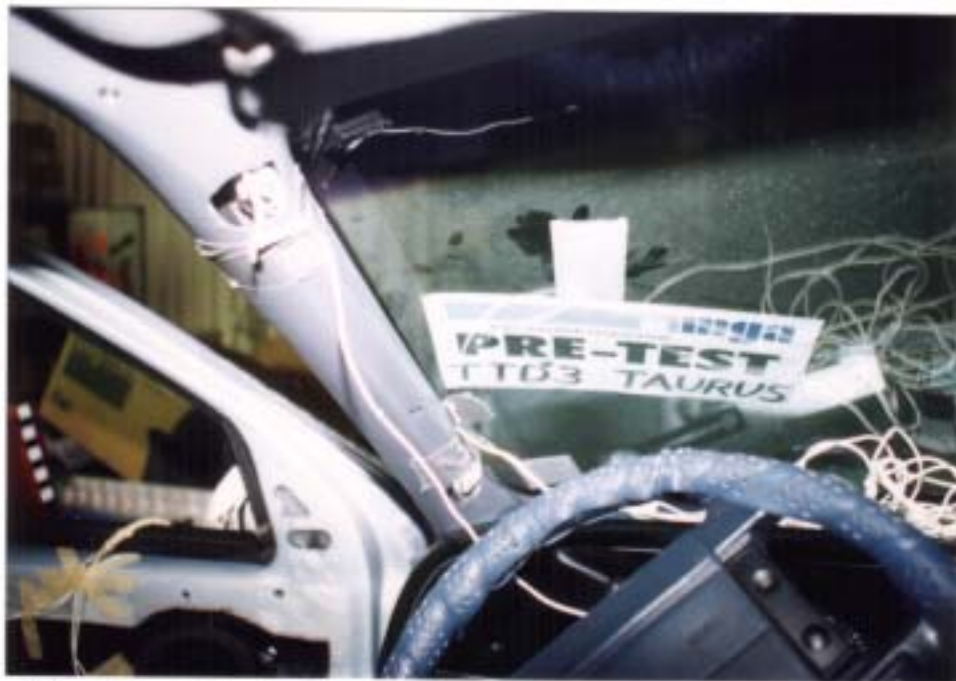
Photo No. A-56 - Pre-Test Left Mid and Upper A-Post Accelerometer
