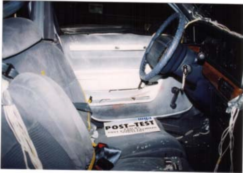
Photo No. A-29 - Post-Test Front Passenger Dummy Contact
