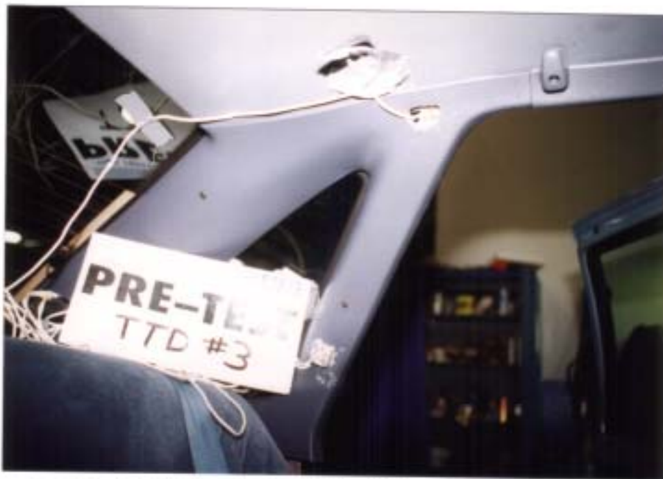
Photo No. A-58 - Pre-Test Left Mid and Upper C-Post Accelerometer
