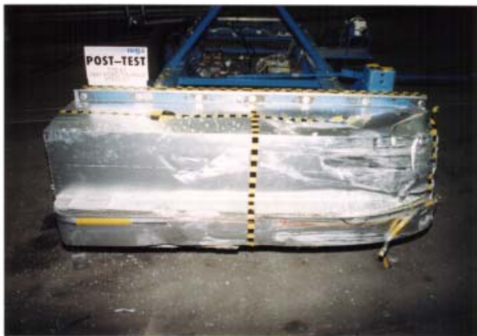
Photo No. A-16 - Post-Test MDB Front View
