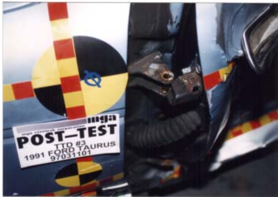
Photo No. A-54 - Post-Test Front Door Upper Hinge Pin Failure
