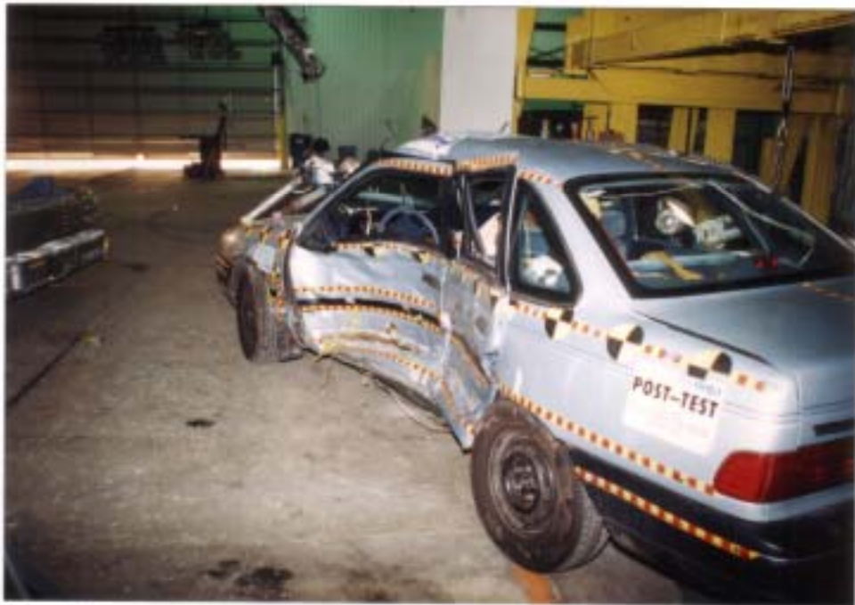
Photo No. A-11 - Post-Test MDB Positioned Against Vehicle (right side)
