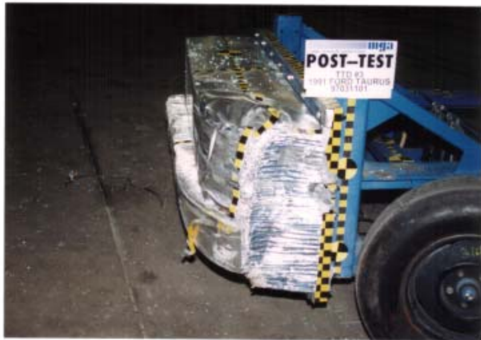
Photo No. A-18 - Post-Test MDB Left Side View
