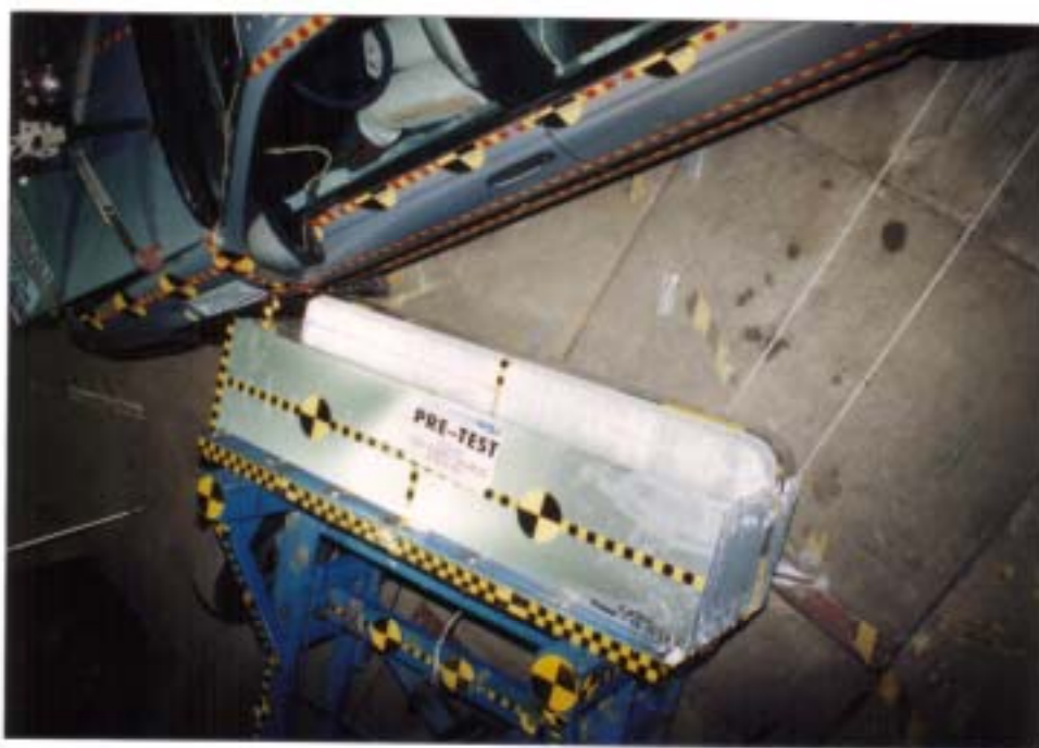
Photo No. A-9 - Pre-Test MDB Positioned Against Vehicle Overhead View
