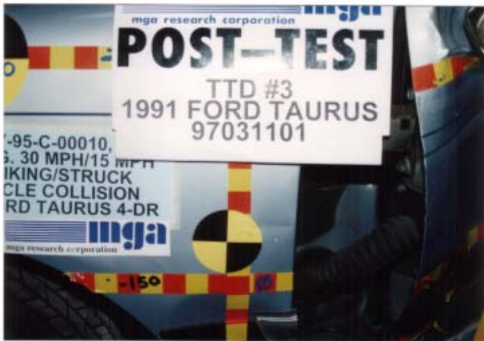
Photo No. A-41 - Post-Test Right Front Impact Point on Vehicle
