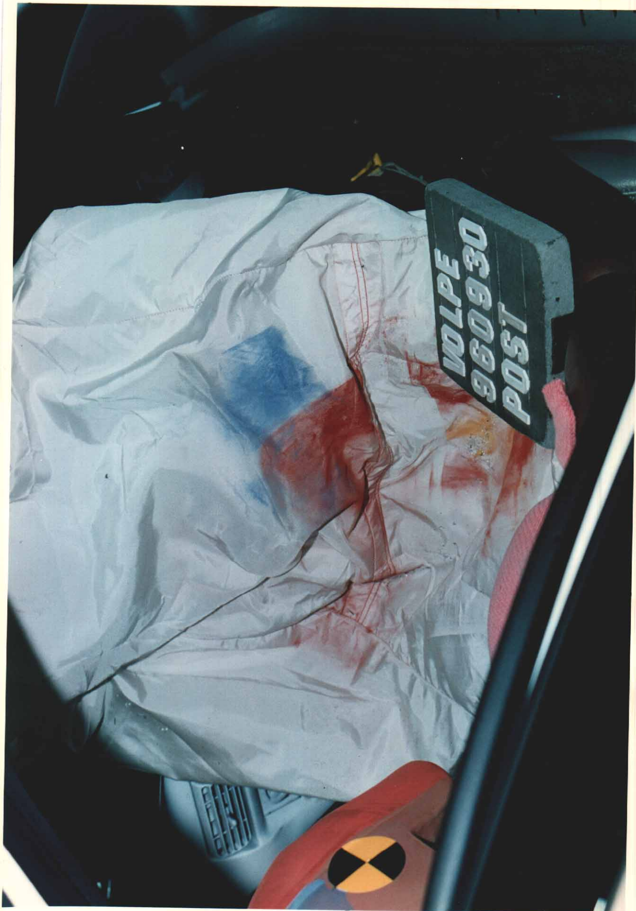
Figure A-44 Post-Test Passenger Dummy Head Contact - View 2
