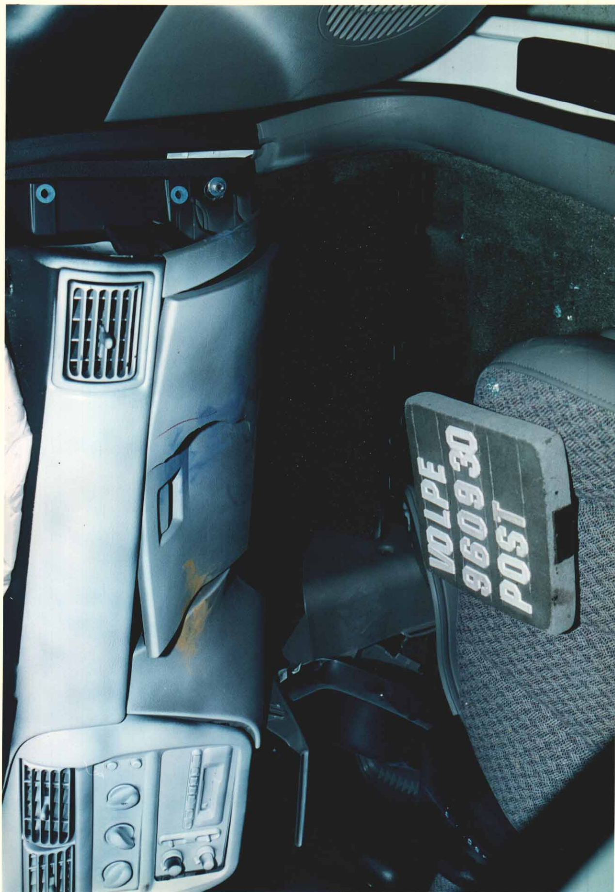
Figure A-47 Post-Test Passenger Dummy Knee Contact - View 2
