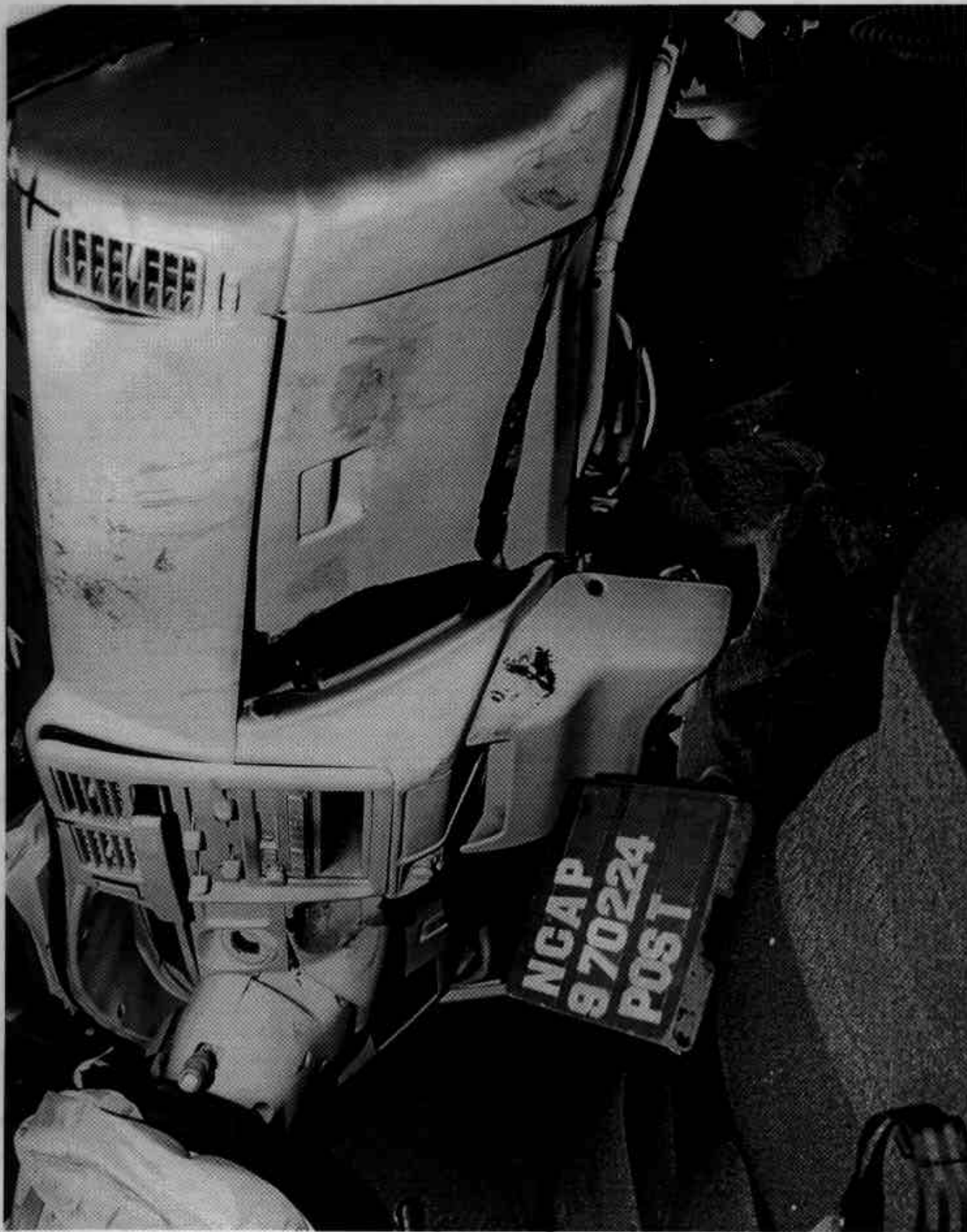
Figure A-49 Post-Test Passenger Dummy Knee Contact - View 1
