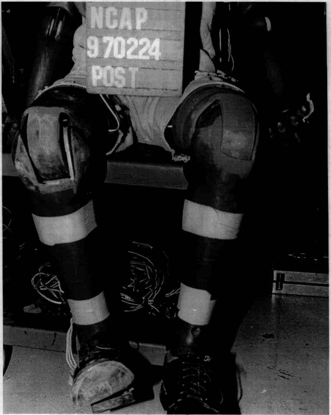
Figure A-46 Post-Test Driver Dummy Knee Contact - View 1
