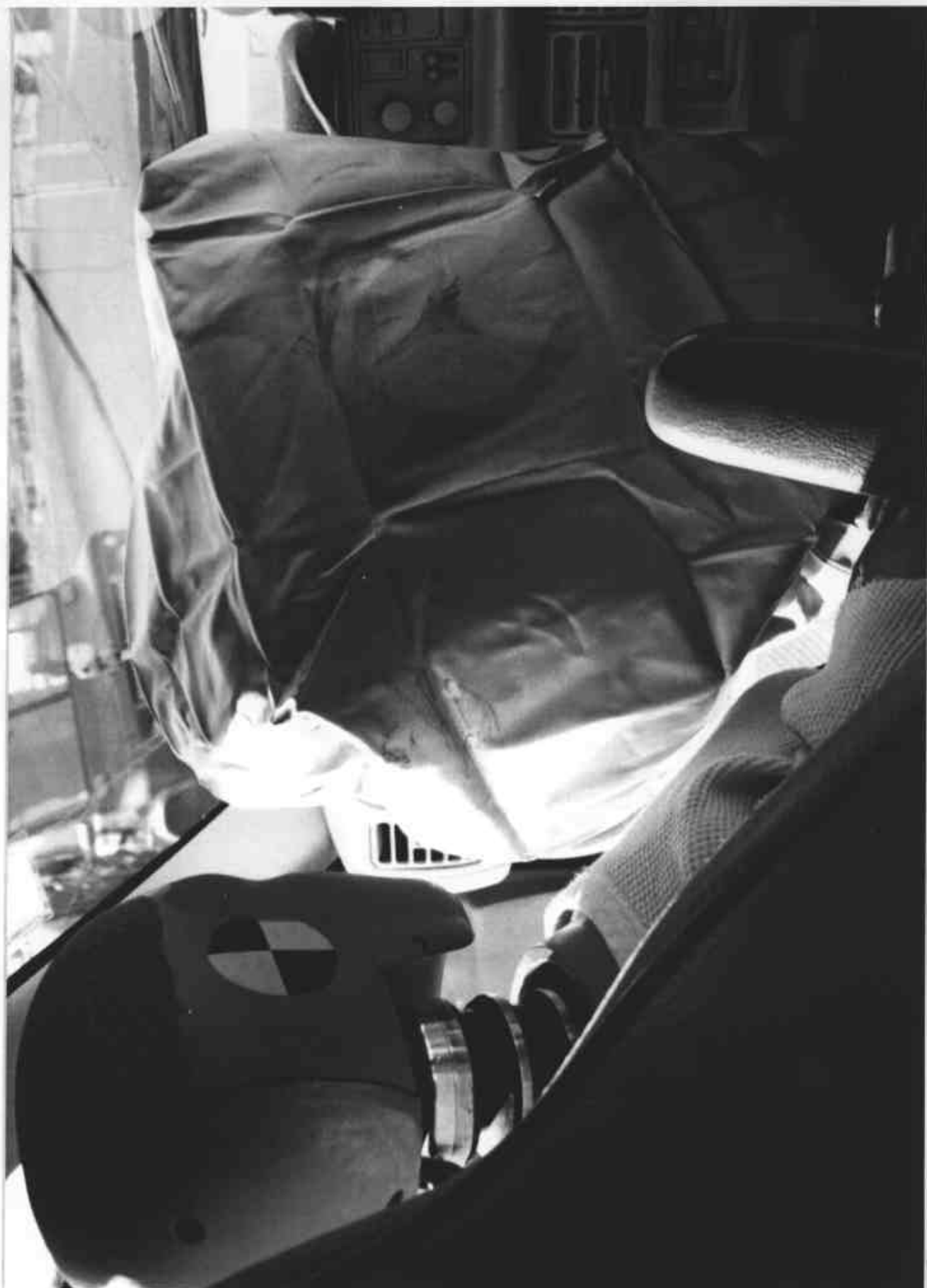
Figure B-29 POST-TEST DRIVER CHEST CONTACT POINT
