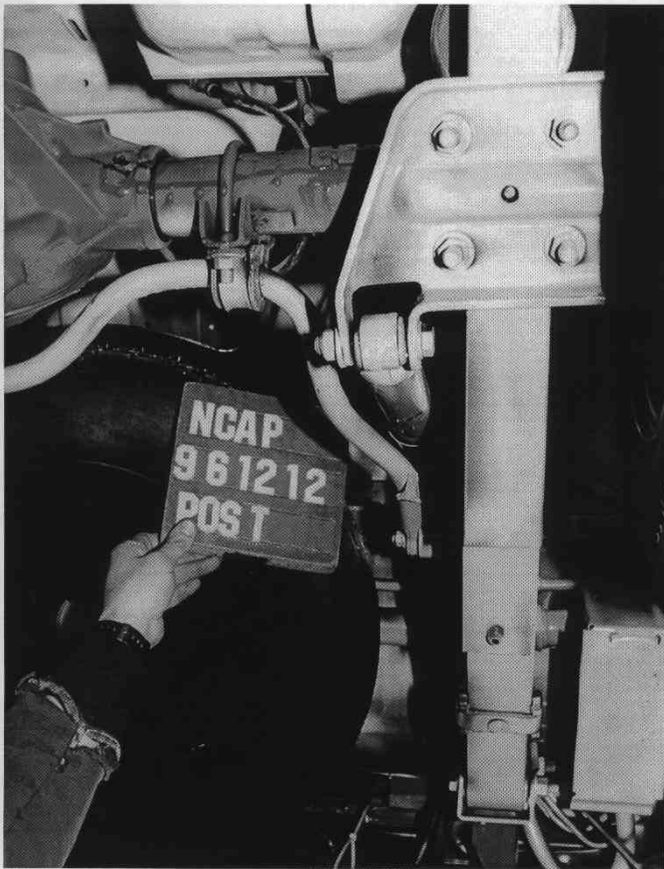
Figure A-21 Post-Test Fuel Filler Neck View
