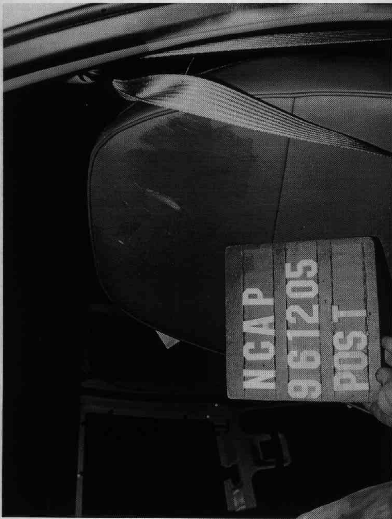
Figure A-43 Post-Test Driver Dummy Head Contact - View 3
