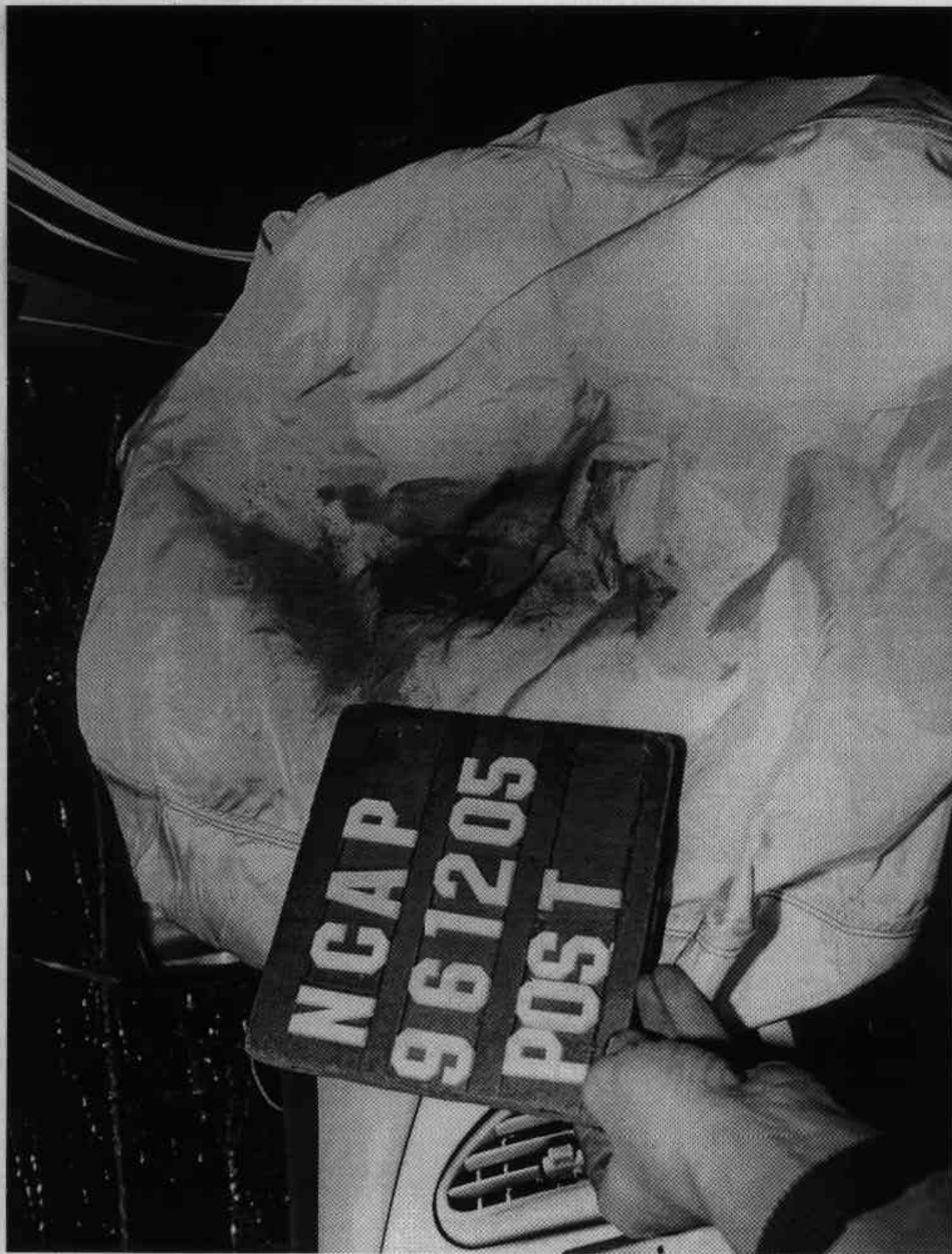
Figure A-47 Post-Test Passenger Dummy Head Contact - View 2
