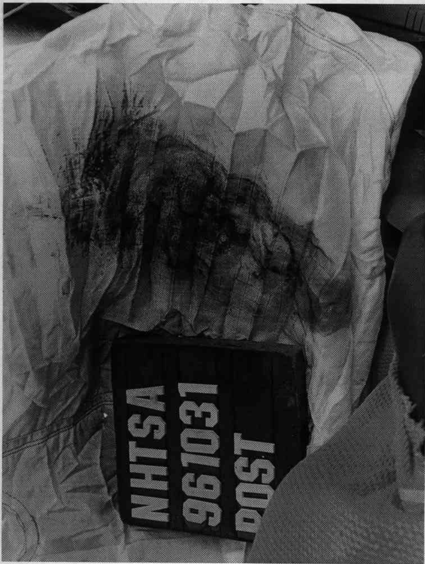
Figure A-21. Post-test Passenger Dummy Head Contact - View 2
