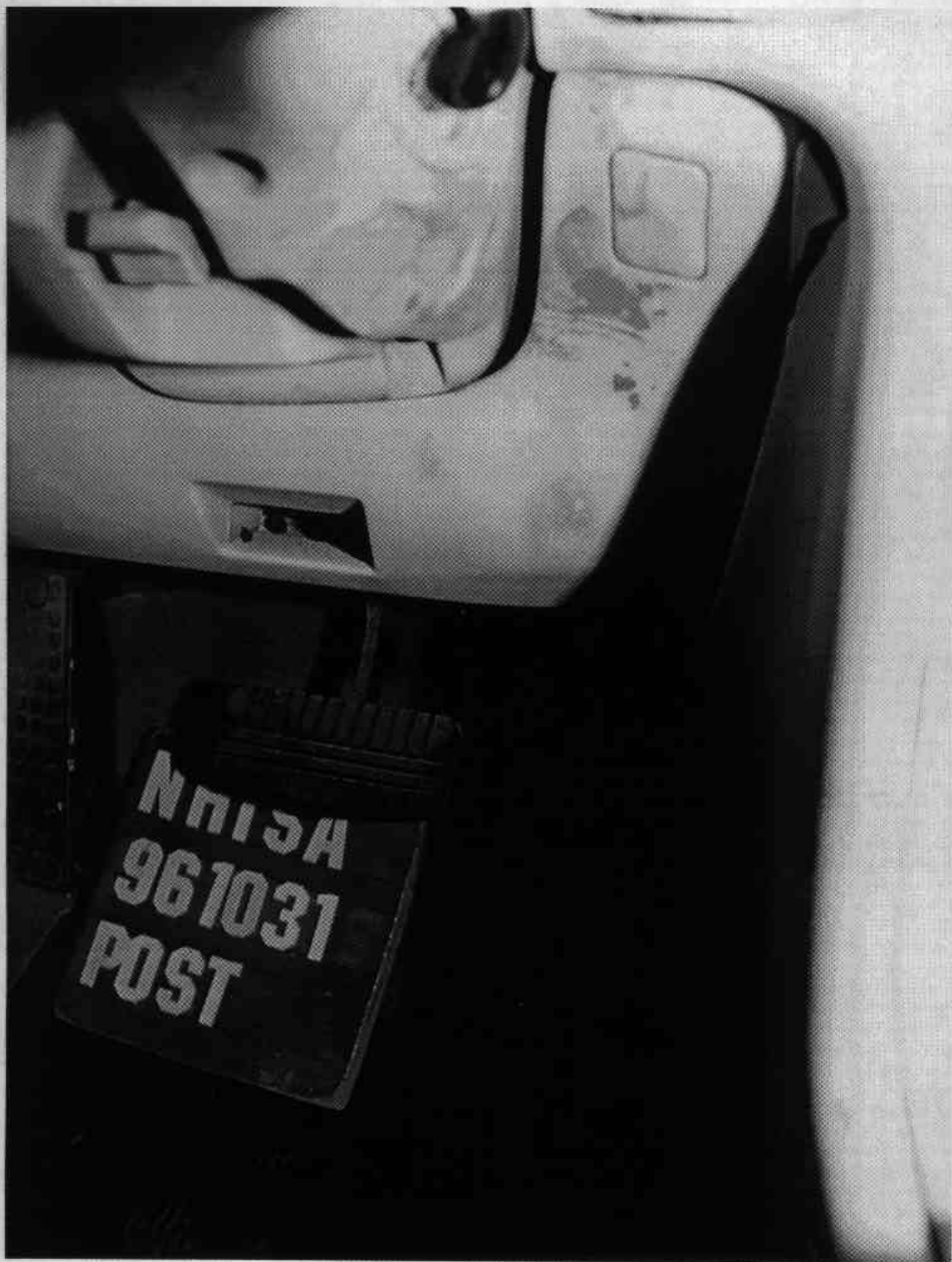
Figure A-19. Post-test Driver Dummy Knee Contact - View 3
