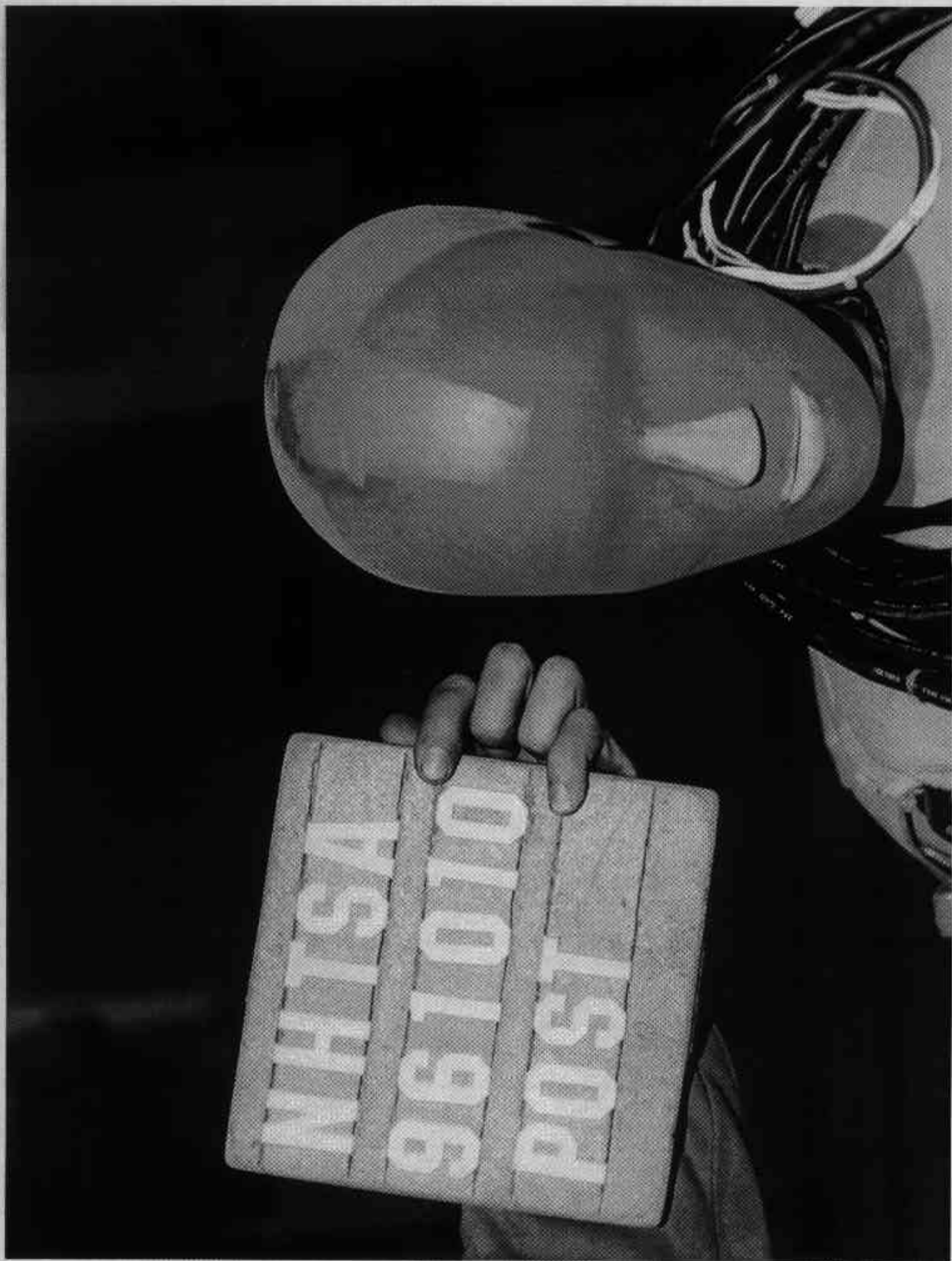
Figure A-19. Post-test Passenger Dummy Head Contact - View 1
