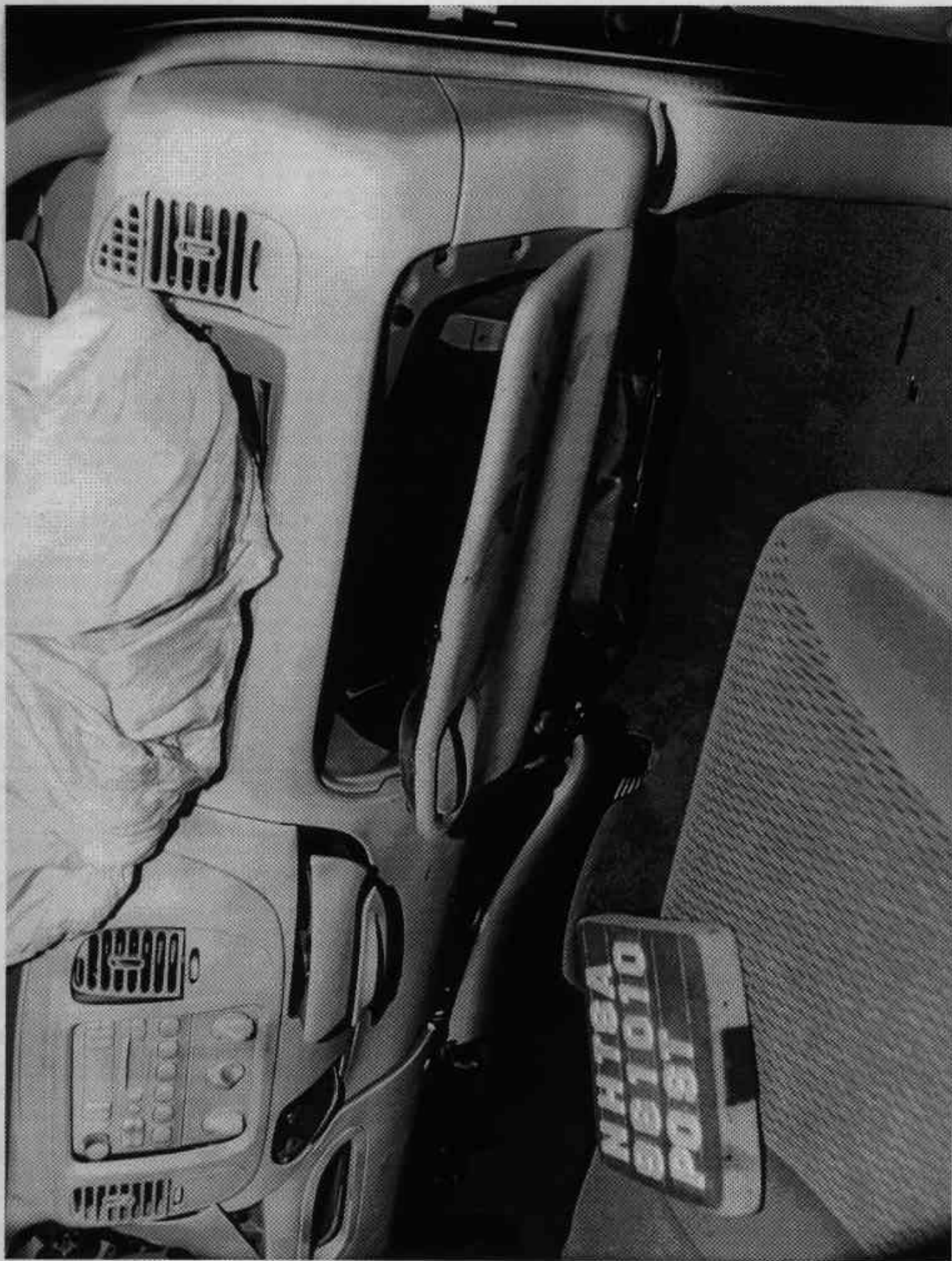
Figure A-22. Post-test Passenger Dummy Knee Contact - View 2
