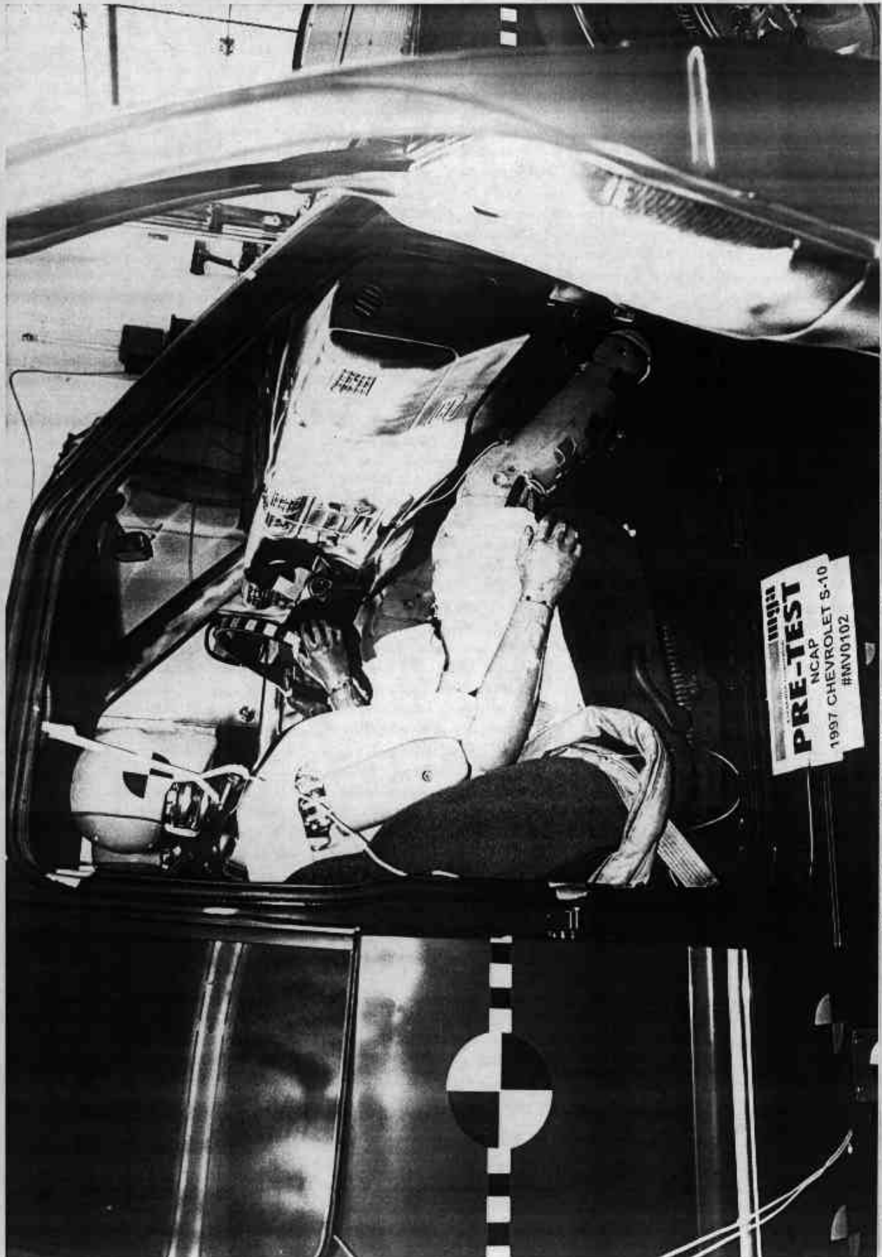
Photo No. A-38 - Pre-Test Passenger Dummy Position Right Side View (Door Open)
