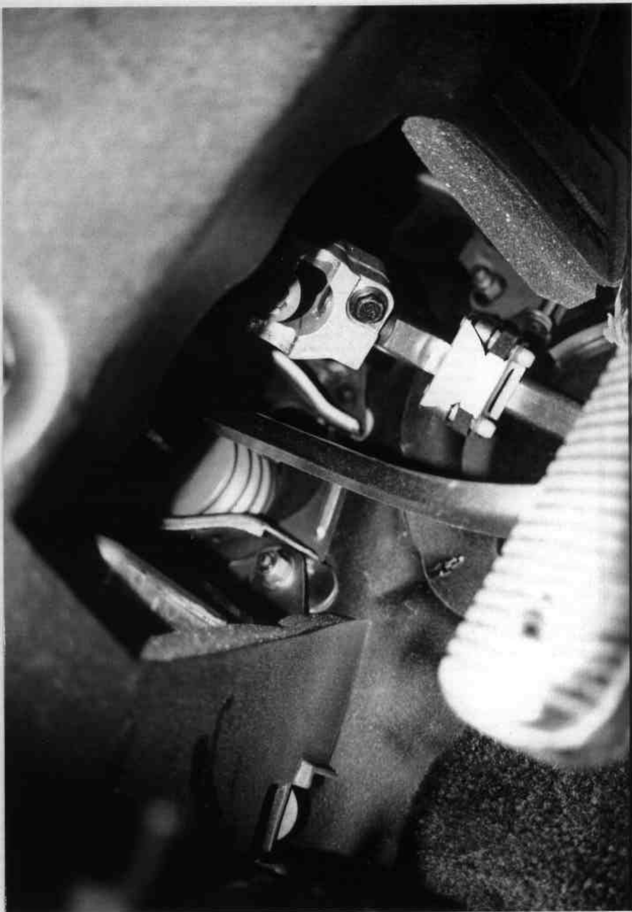
Figure A-20 POST-TEST STEERING COLUMN/FIREWALL INSIDE VIEW
