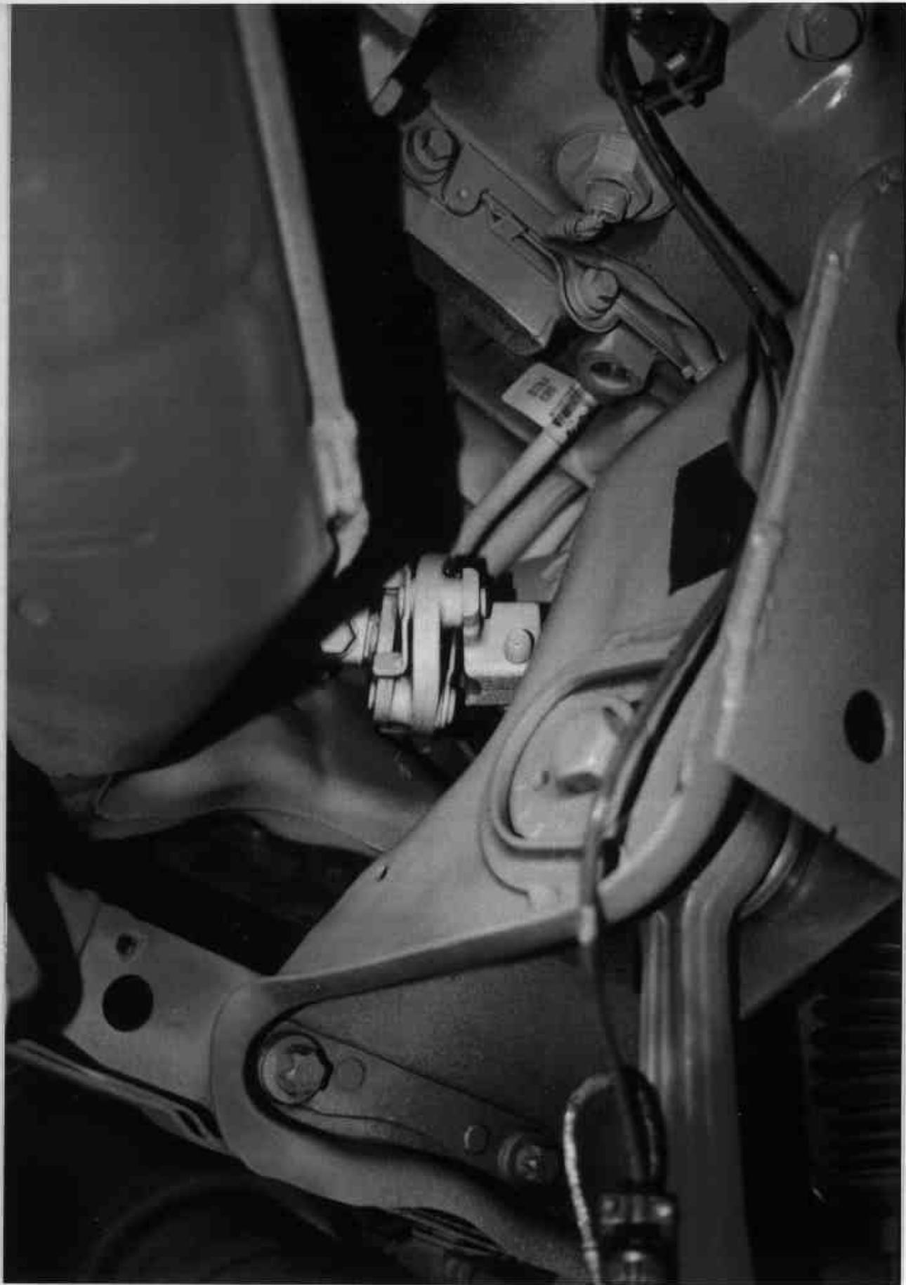
Figure A-17 PRE-TEST UNDERBODY STEERING SHAFT
