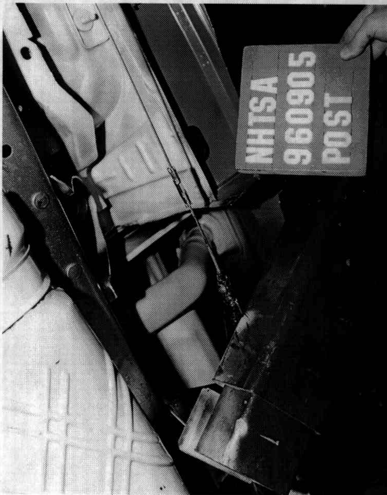
Figure A-20 Post-Test Fuel Filler Neck View
