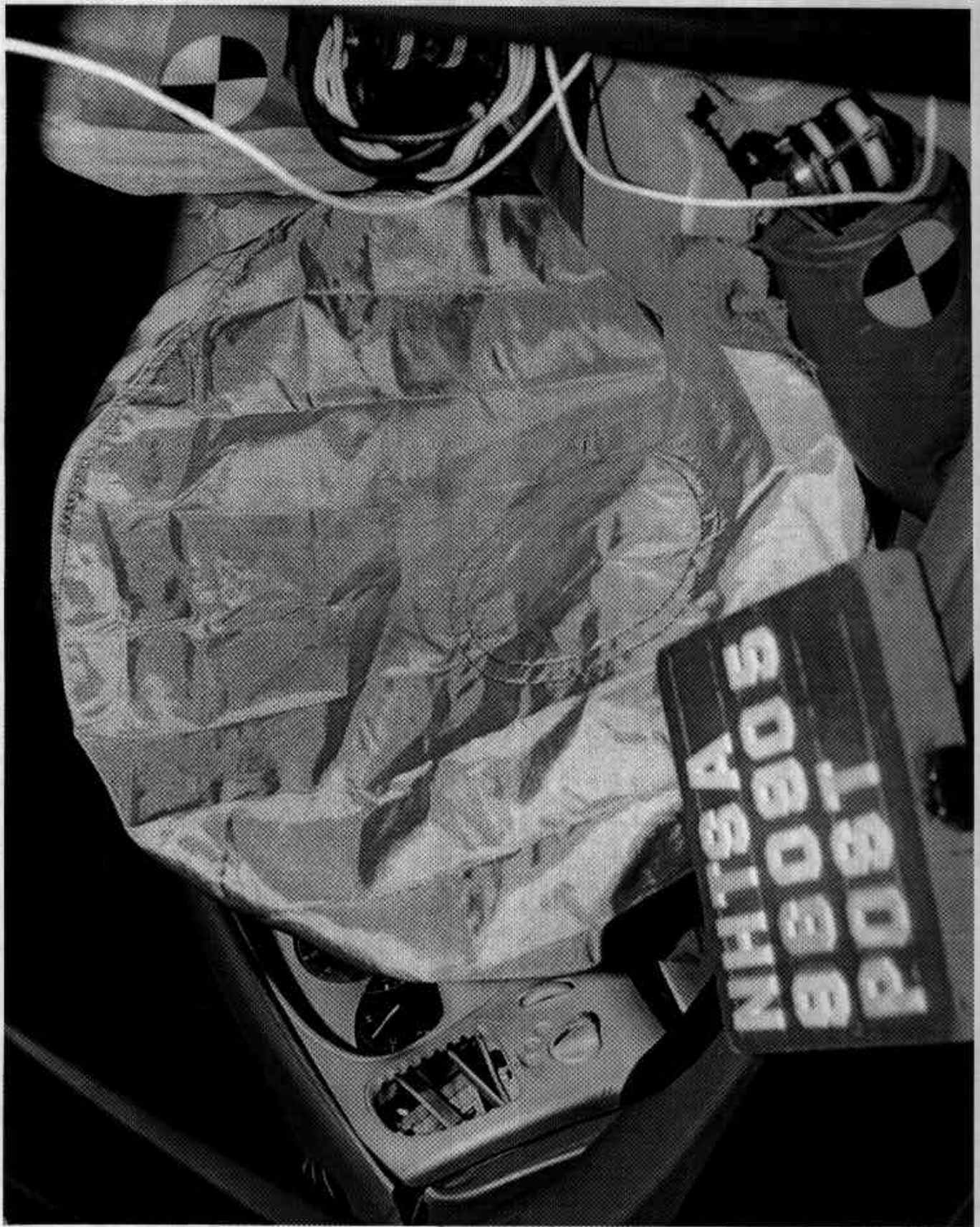
Figure A-40 Post-Test Driver Dummy Head Contact - View 2
