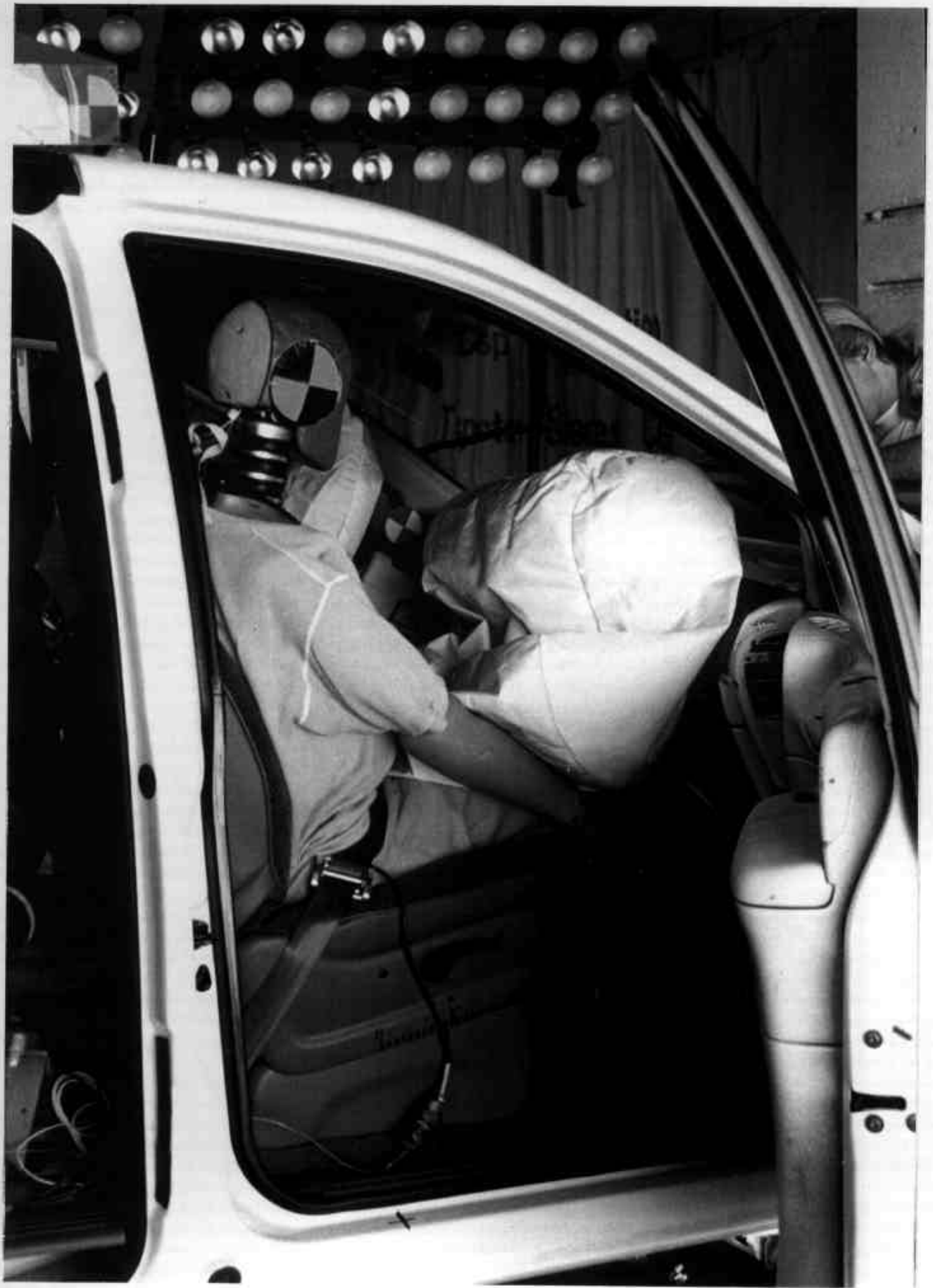
Figure A-29 POST-TEST PASSENGER AND INTERIOR VIEW A-32
