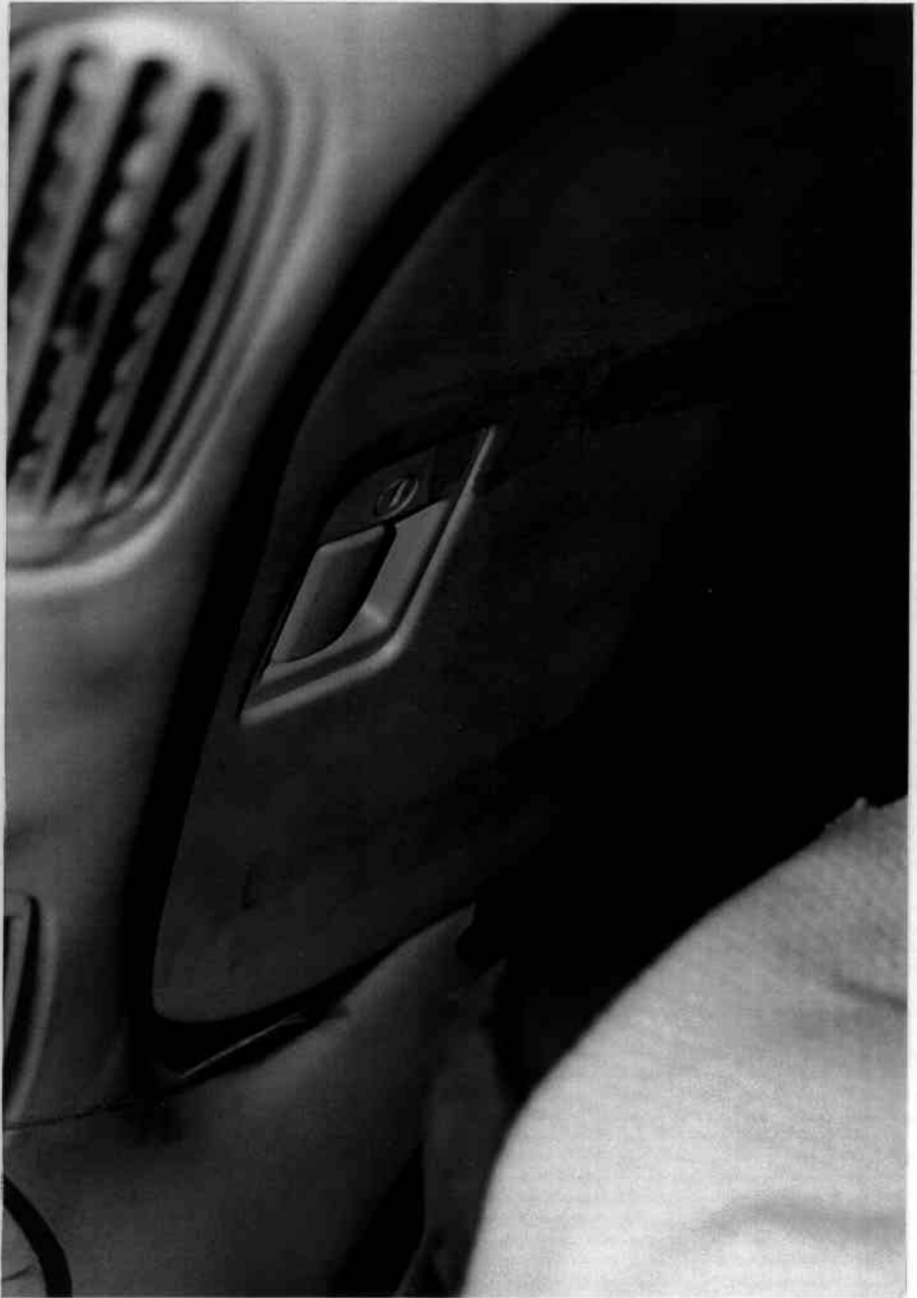
Figure A-16 POST-TEST PASSENGER KNEE BOLSTER
