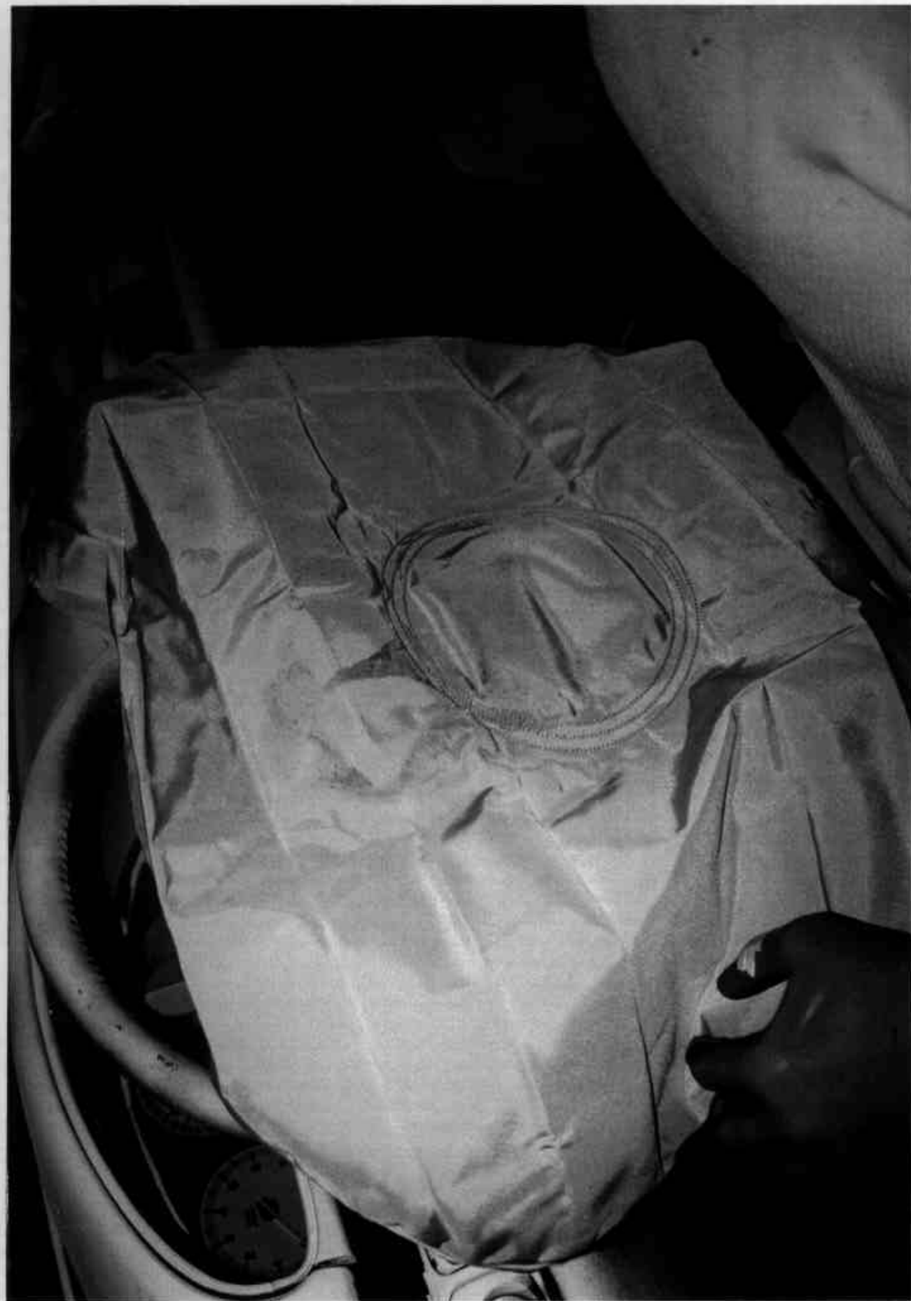
Figure A-24 POST-TEST DRIVER AIRBAG VIEW
