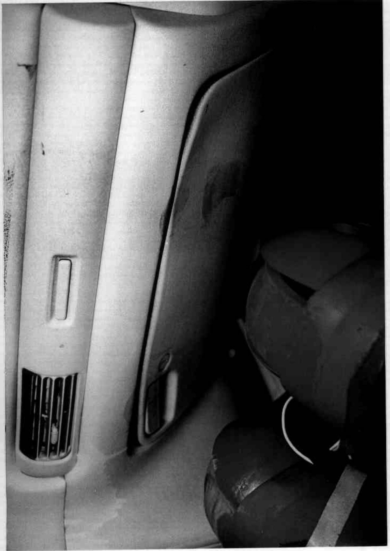
Figure A-16 POST-TEST PASSENGER KNEE BOLSTER
