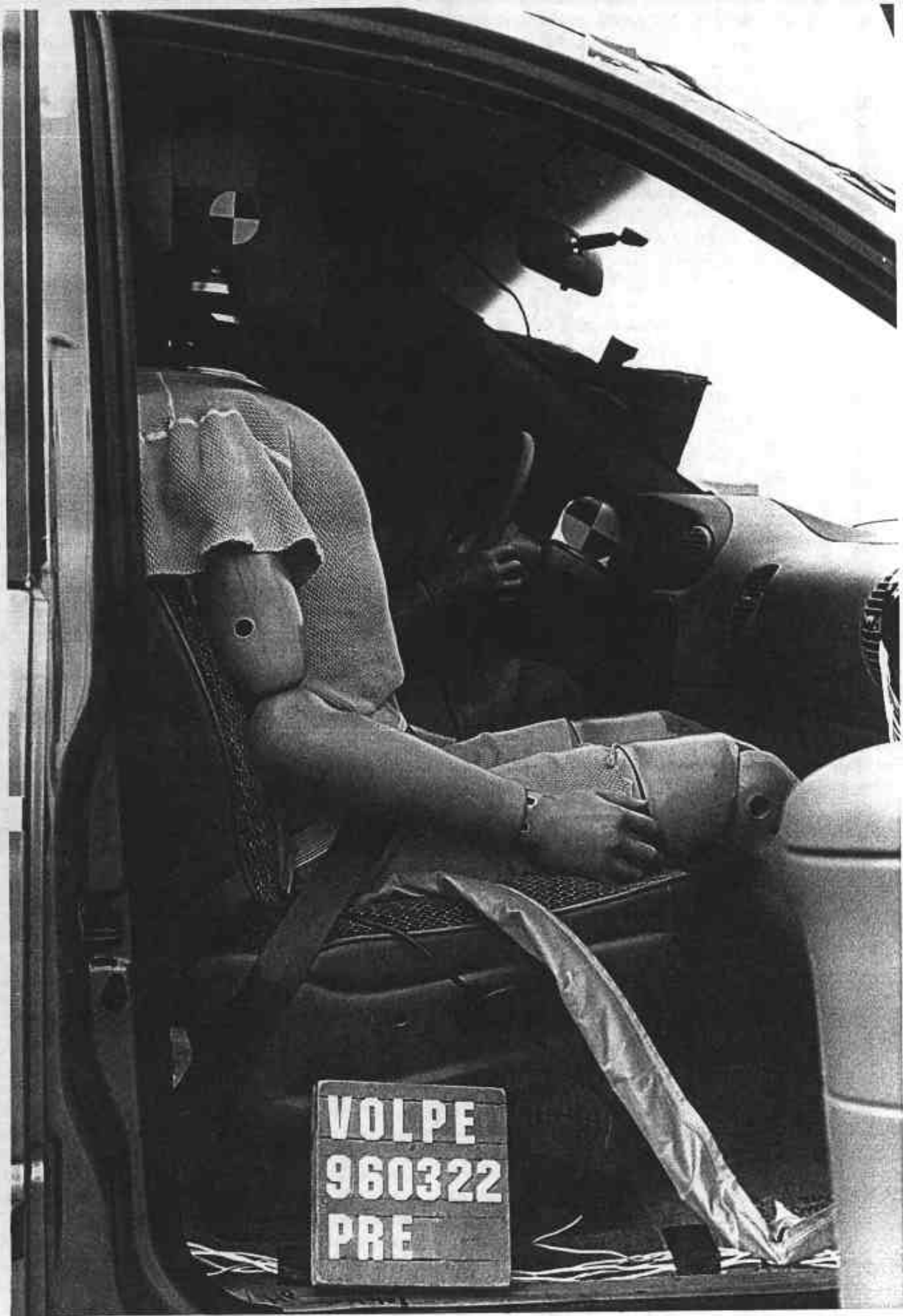
Figure A-32 Pre-Test Passenger Dummy and Vehicle Interior - View 2
