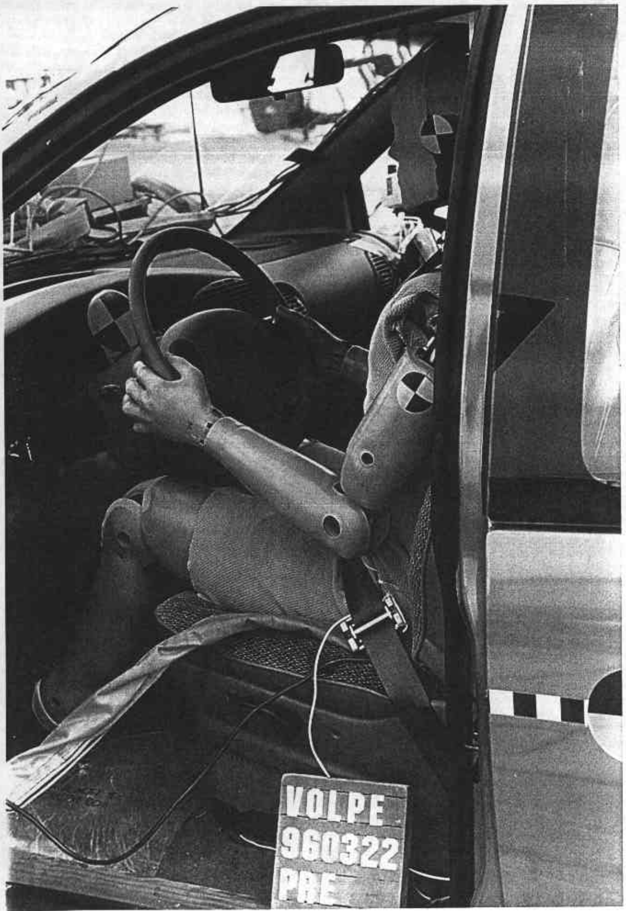
Figure A-26 Pre-Test Driver Dummy and Vehicle Interior - View 1
