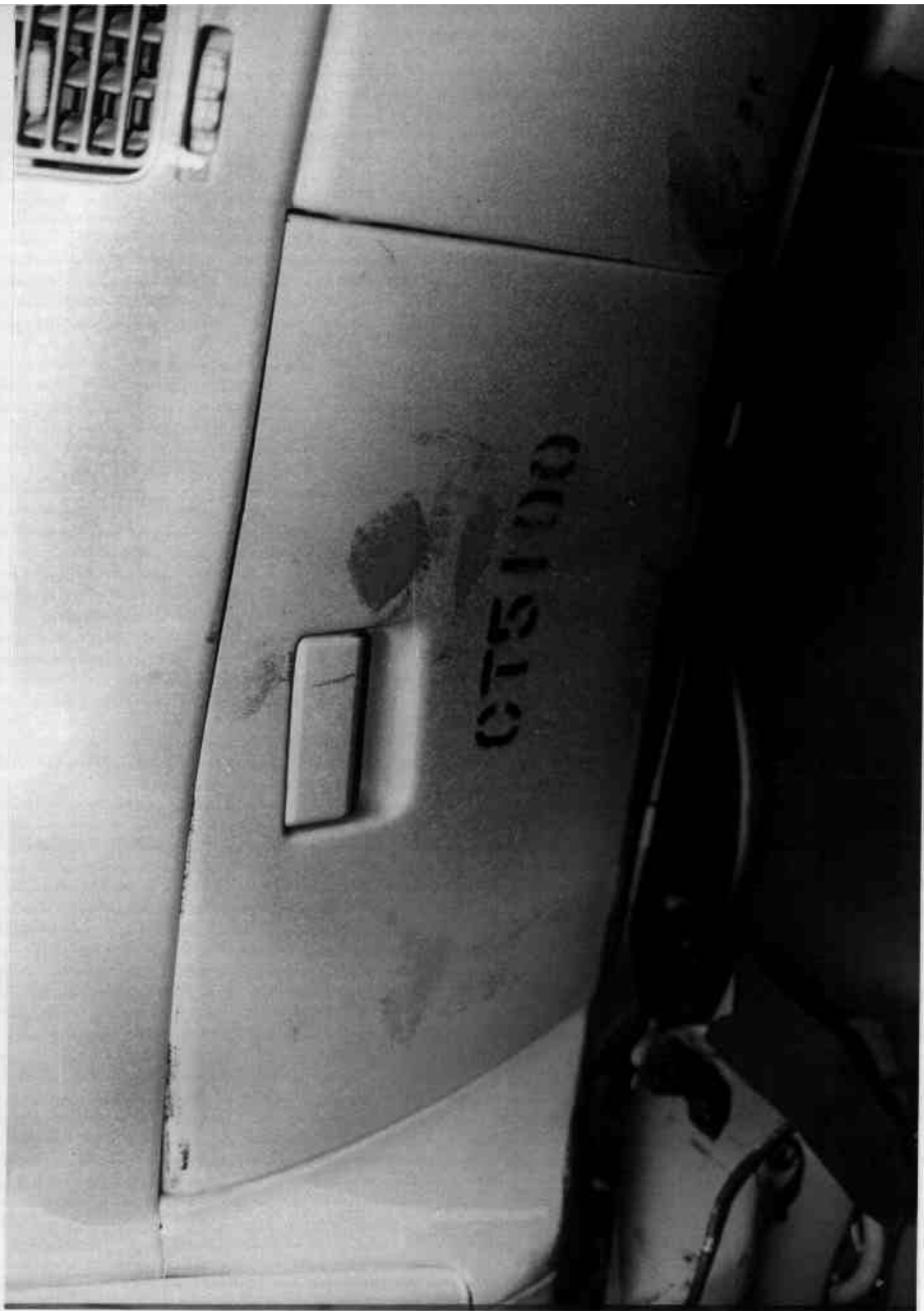
Figure A-16 POST-TEST PASSENGER KNEE BOLSTER
