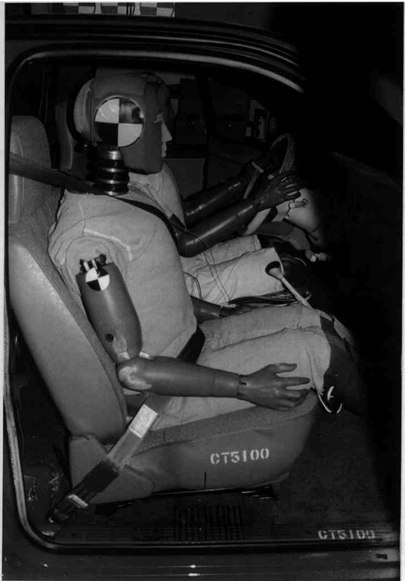
Figure A-11 PRE-TEST PASSENGER SIDE VIEW A-13
