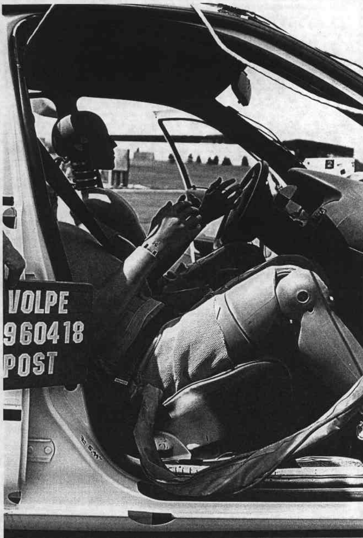
Figure A-38 Post-Test Passenger Dummy & Vehicle Interior - View 1
