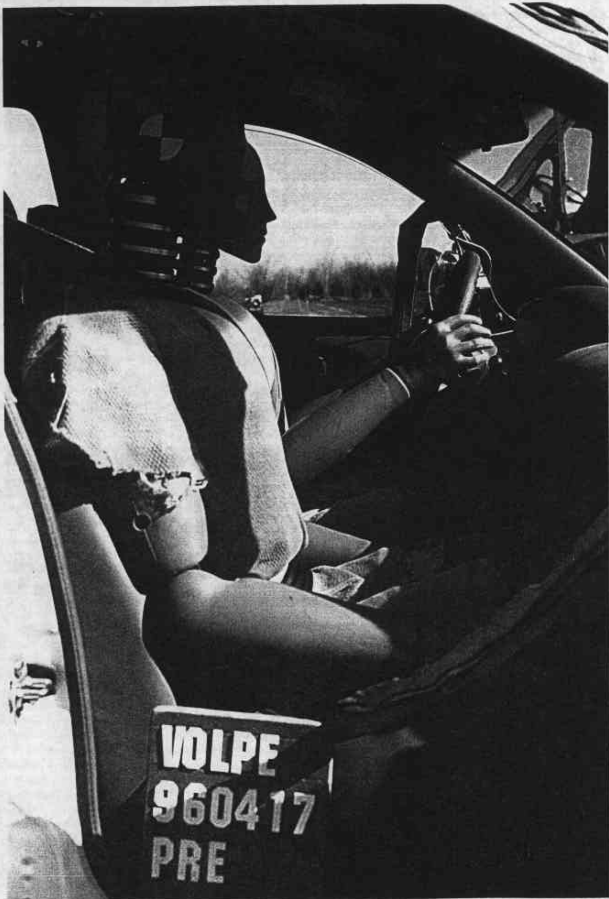
Figure A-38 Pre-Test Passenger Dummy & Vehicle Interior - View 1
