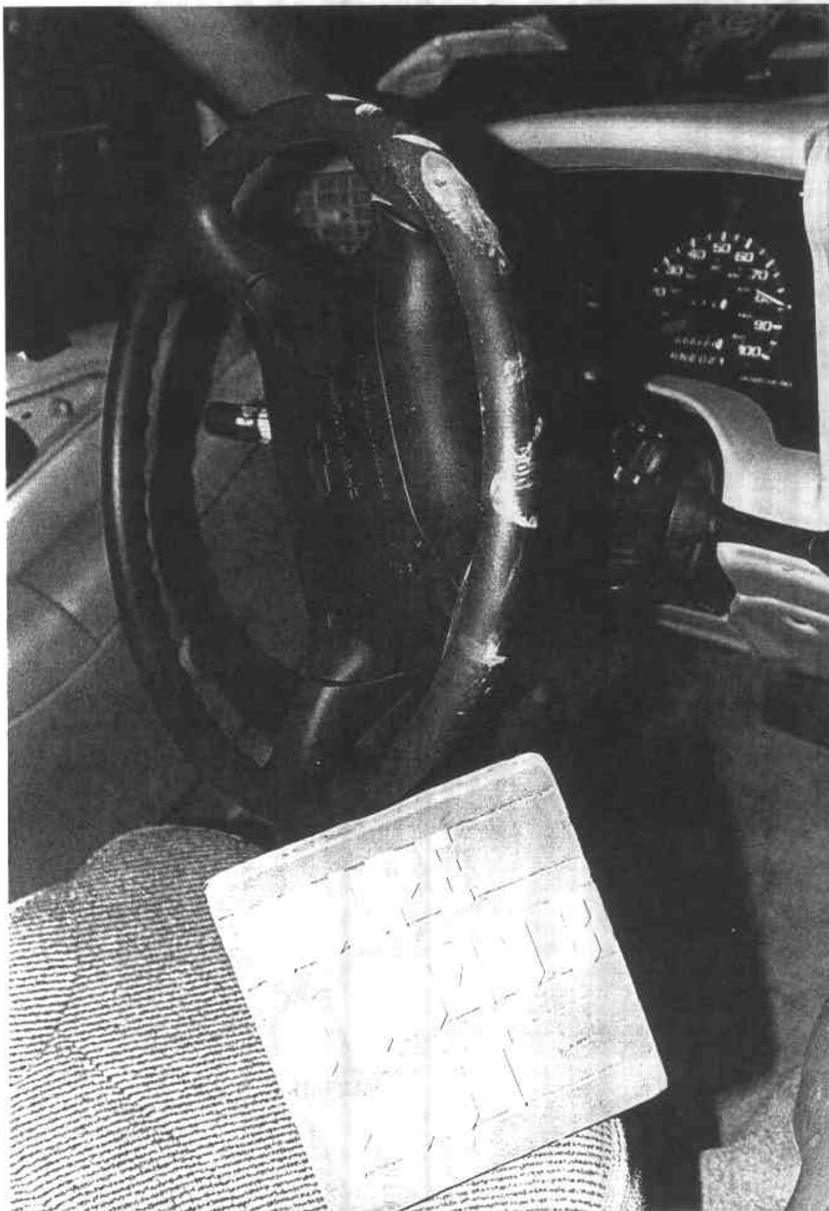
Figure A-45 Post-Test Driver Dummy Knee Contact - View 2
