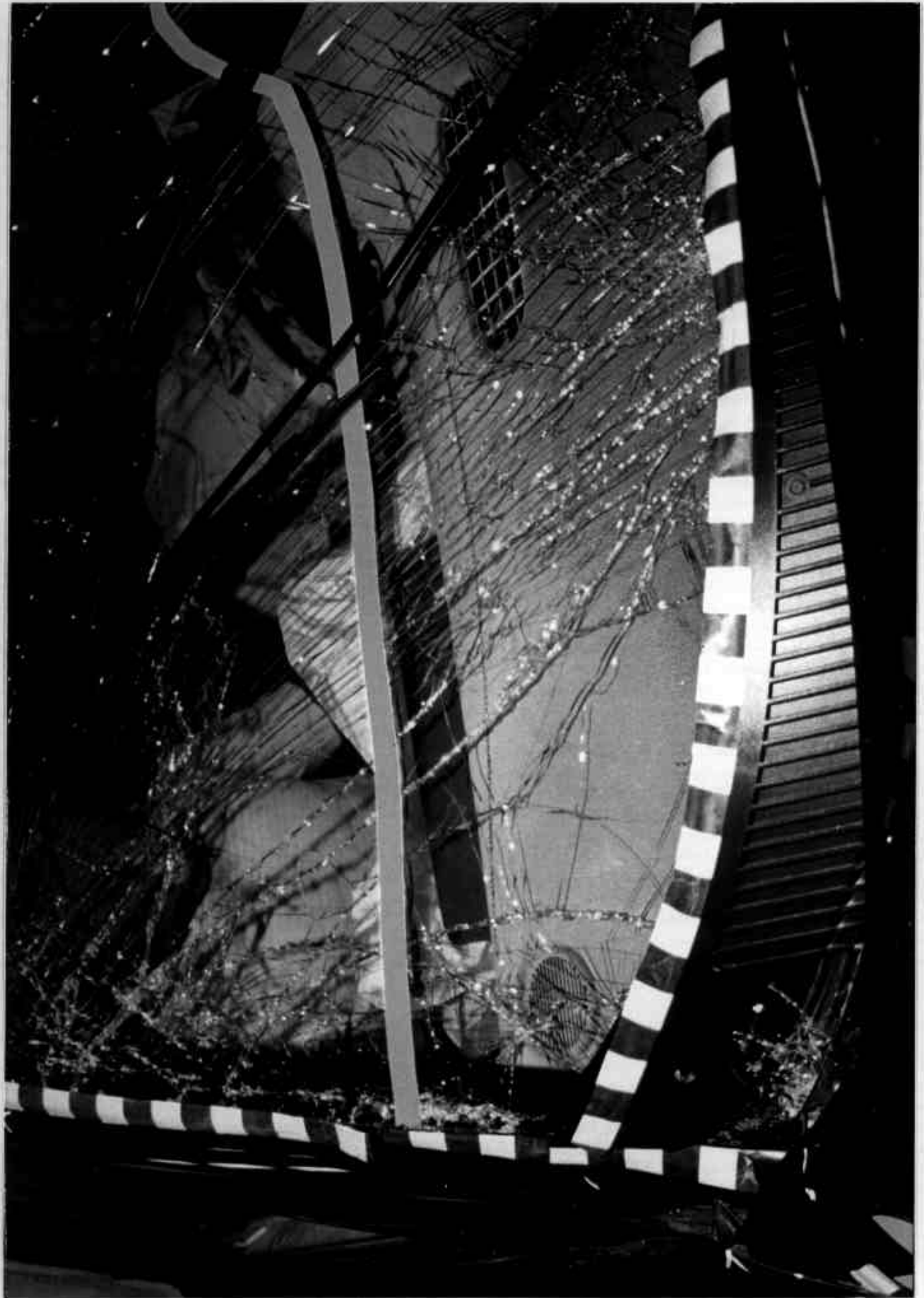
Figure A-52 POST-TEST FRONT SIDE OF WINDSHIELD RETENTION LOSS
