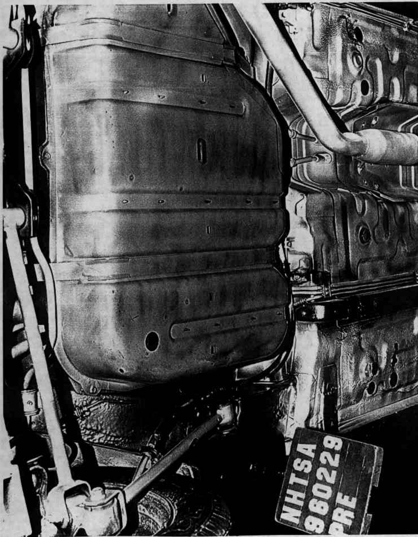
Figure A-21 Pre-Test Fuel Tank View
