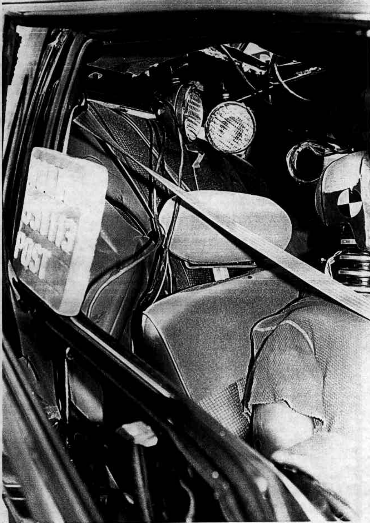
Figure A-45. Post-Test Passenger Dummy Head Contact - View 2 A-46
