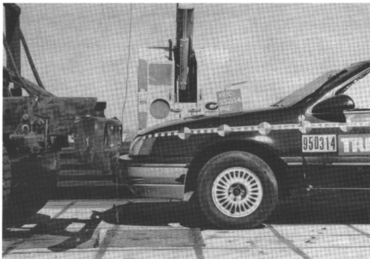
Figure A-25 Pre-Test Bumper Engagement - View 1
