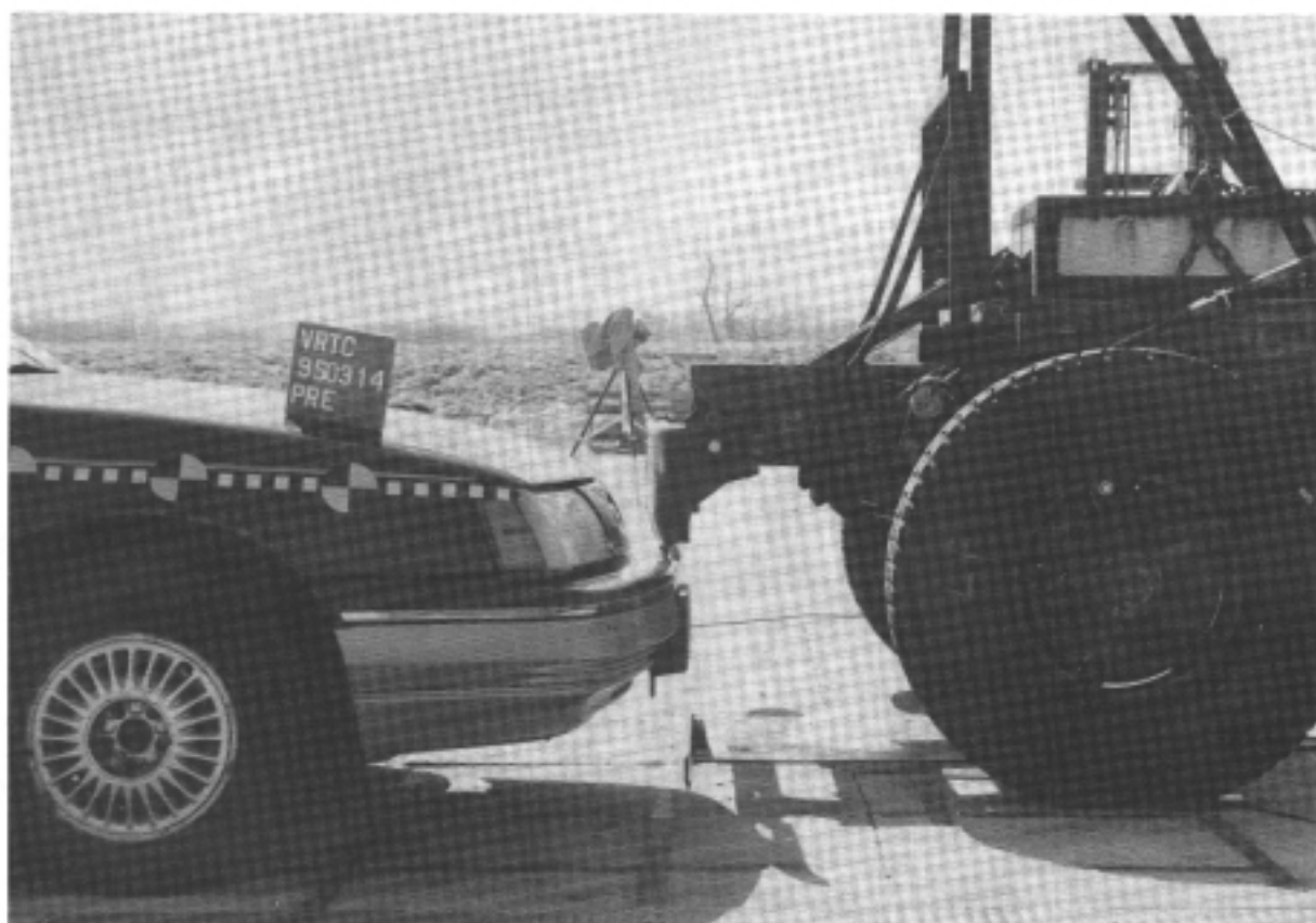
Figure A-26 Pre-Test Bumper Engagement - View 2
