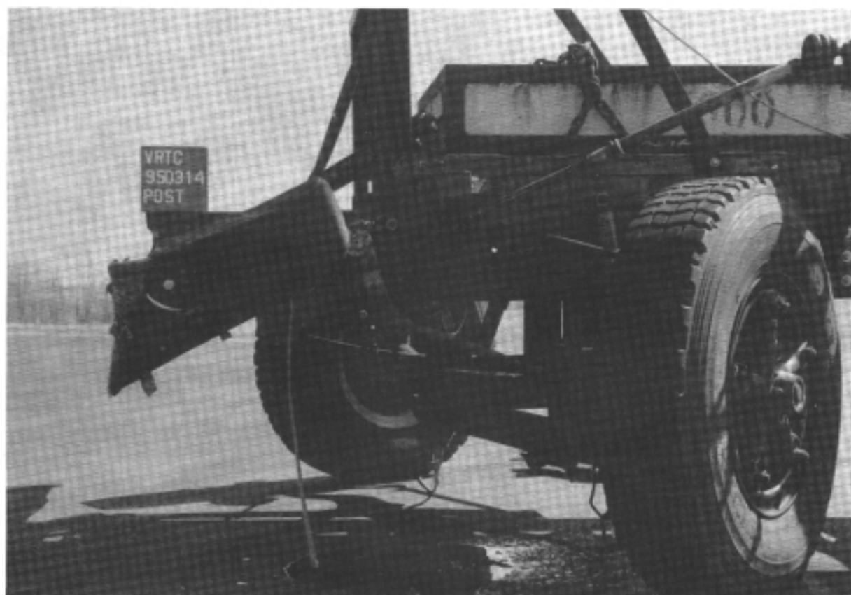
Figure A-30 Post-Test Truck Damage - View 2
